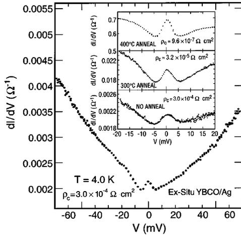
FIG. 1. Conductance  $dI/dV$  as a function of bias voltage  $V$  for a planar,  $c$ -axis YBCO/Ag interface ( $\sim 8 \times \sim 8 \mu\text{m}$ ) formed *ex situ*, that is, after exposing the YBCO surface to air. Inset: Low-bias data indicating the similarity of the zero-bias conductance peak after exposing the interface to 30-min oxygen anneals at progressively higher temperature.
