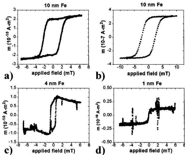
FIG. 2. (a), (c), (d) Hysteresis loops of integrated  $m$  vs  $B_0$  for iron films measured with the MTM. (b) A typical hysteresis loop of integrated  $m$  vs  $B_0$  for iron films measured with the AGM.
