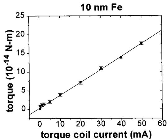
FIG. 3. Torque vs torque coil current for an iron film thickness of 10 nm.
