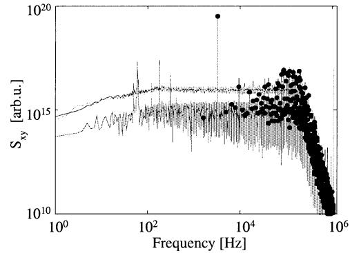
Fig. 5. Power spectra on a log-log scale of a QVNS synthesized sine wave. The upper two curves are noise spectra for each of the amplifier chains. The lower curve is the cross-correlated power spectrum. Black dots decorate the harmonics of the repetition frequency of the digital code.
