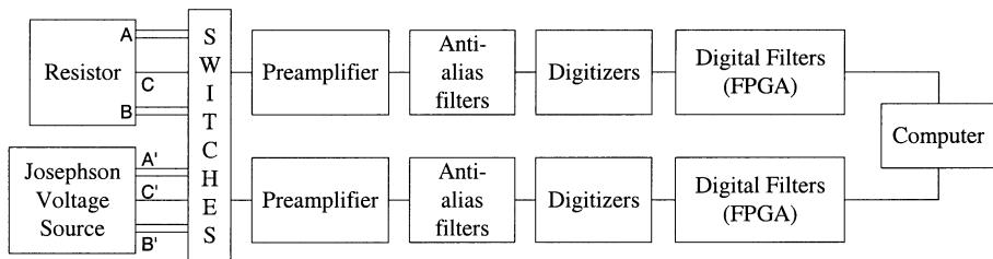
Fig. 1. Block diagram of the Johnson noise thermometry system. For both the resistor and the quantized (Josephson) voltage noise source, we use a five-wire (two signal pairs, A and B, and a common line, C) connection to the preamplifiers. The entire electronic system is battery-powered except for the computer. Connections to the computers are made with optical fibers.
