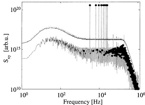
Fig. 6. Power spectra of a QVNS synthesized waveform of eight tones. The upper two curves are noise spectra for each of the amplifier chains. The lower curve is the cross-correlated power spectrum. Black dots decorate the harmonics of the repetition frequency of the digital code.
