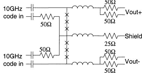
Fig. 3. Schematic of the QVNS. Xs represent Josephson junctions. The input capacitors are inner and outer dc blocks with cutoff frequencies from 10 to 250 MHz.
