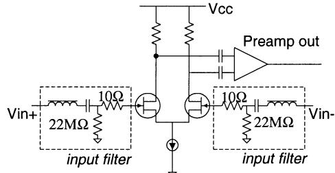
Fig. 4. Schematic of the preamplifier. An optional input filter is used to filter rf noise and remove dc offsets. The input inductor represents a ferrite bead impedance.
