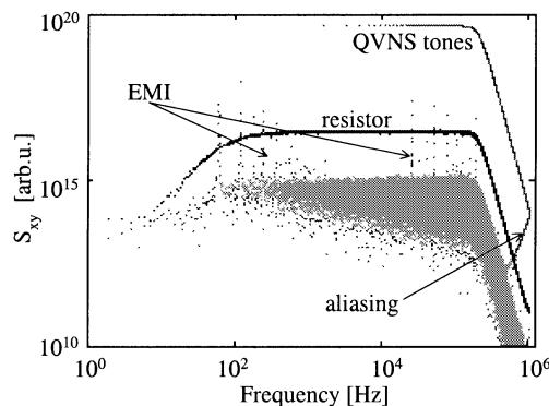
Fig. 7. Cross-correlation spectra of a QVNS pseudo-noise waveform and a 100- $\Omega$  resistor at the Ga triple-point. Each point represents a  $\sim 1$ -Hz frequency bin. The electromagnetic interference (EMI) in this measurement is indicated by arrows.
