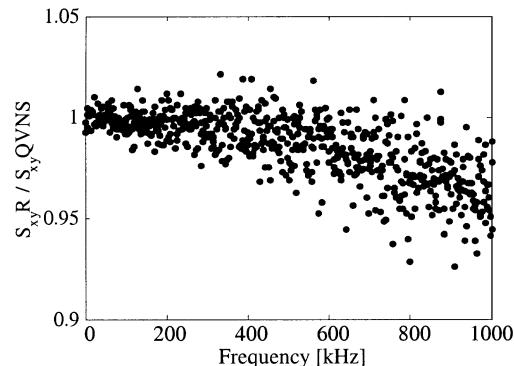
Fig. 8. Ratio of the cross-correlation spectra from the 100- $\Omega$  resistor at the Ga triple-point to the QVNS as a function of the tone frequencies in the QVNS waveform.
