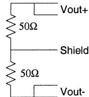
Fig. 2. Schematic of the five-wire connection to a  $100\text{-}\Omega$  resistance.
