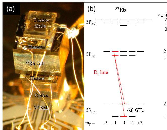
Fig. 1. (a) Picture of the  $^{87}\text{Rb}$  D<sub>1</sub> CSAC physics package. (b) Level diagram of  $^{87}\text{Rb}$ .
