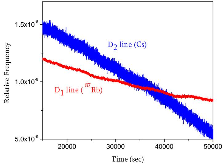
Fig. 3. Measured clock frequency normalized to the hyperfine frequency as a function of time for the  $^{87}\text{Rb}$   $D_1$  CSAC (red). It can be seen that the slow frequency drift is reduced compared to the first Cs  $D_2$  CSAC (blue).
