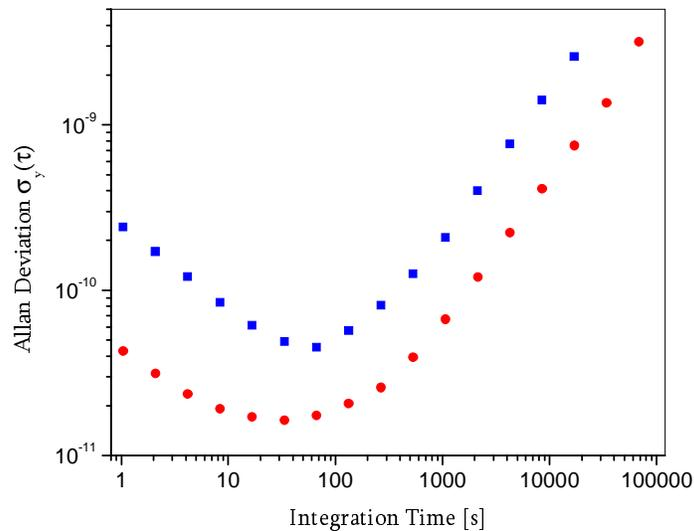
Fig. 2. Measured Allan deviation for the <sup>87</sup>Rb D<sub>1</sub> CSAC (red dots). It shows a clear improvement in stability over the first CSAC [1], which was based on the Cs D<sub>2</sub> line (blue squares).
