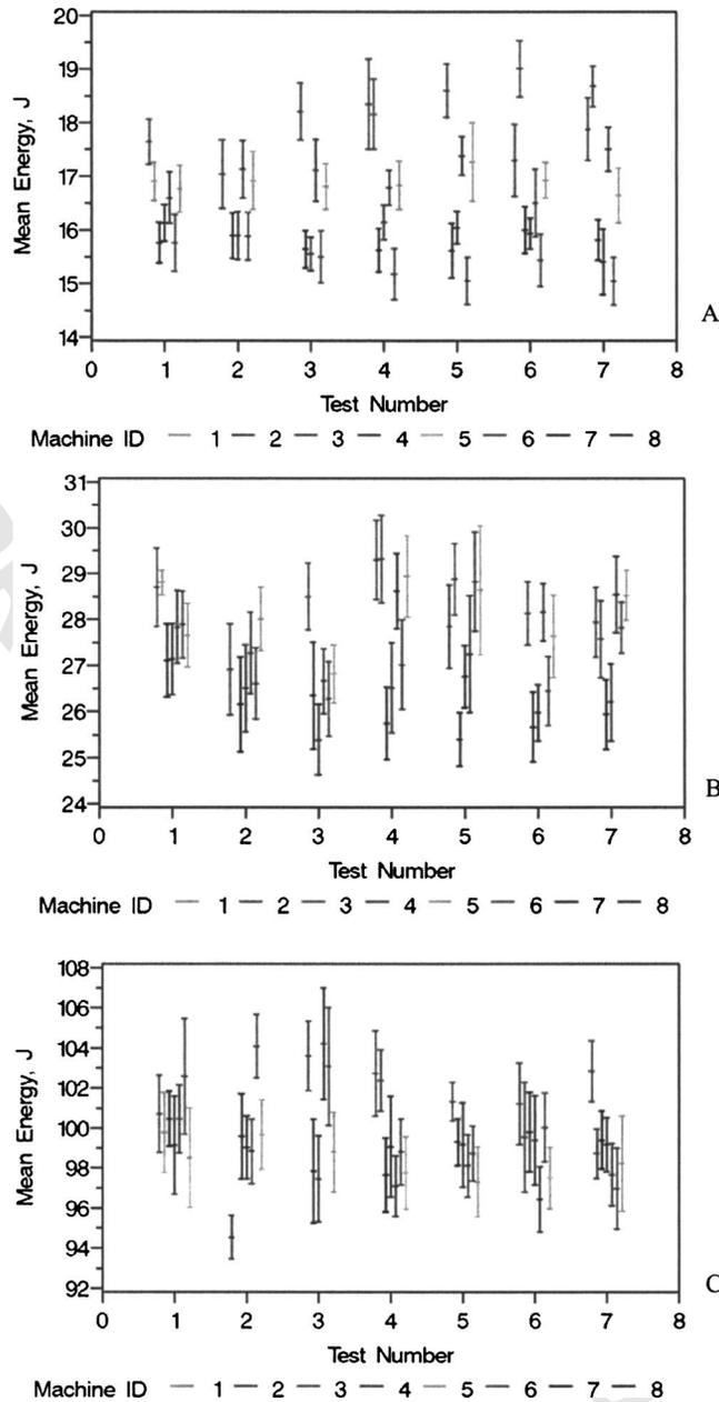
FIG. 2—The average energy for each machine versus test number for: (A) low energy, (B) medium energy, and (C) high energy. Error bars are twice the standard deviation of the mean.
