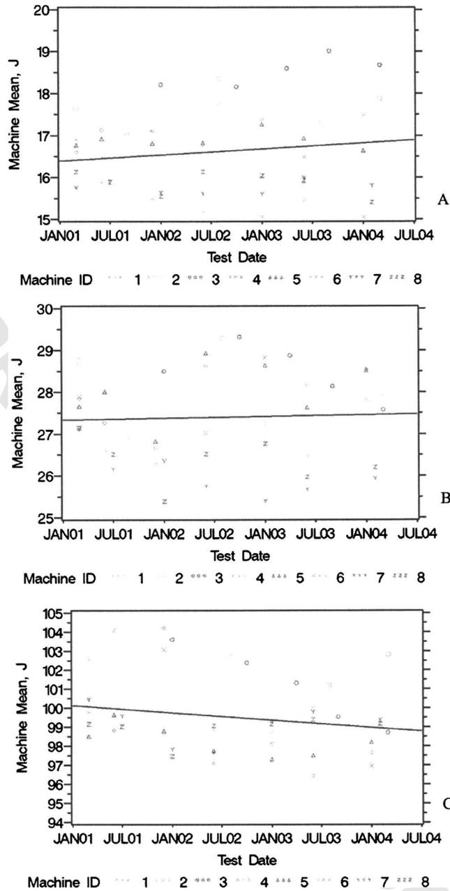
FIG. 1—The (A) low  $p=0.4$ , (B) medium  $p=0.8$ , and (C) high energy  $p=0.2$  plots and probabilities showing trends for specimen stability.
