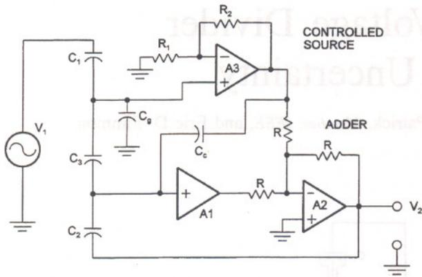
Fig. 2. Implementation of controlled source in active divider.
