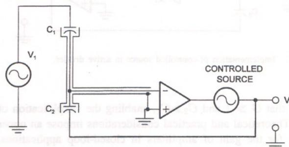
Fig. 1. Active divider with controlled source.
