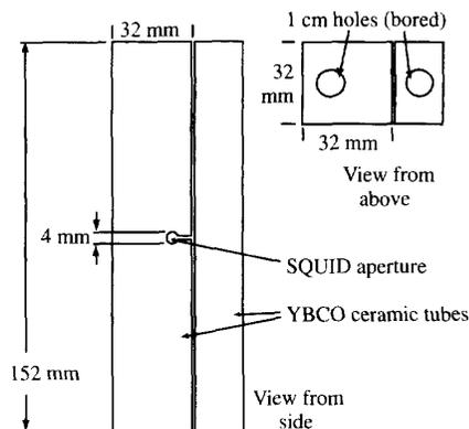
Fig. 2. YBCO tubes in the CCC configuration.
