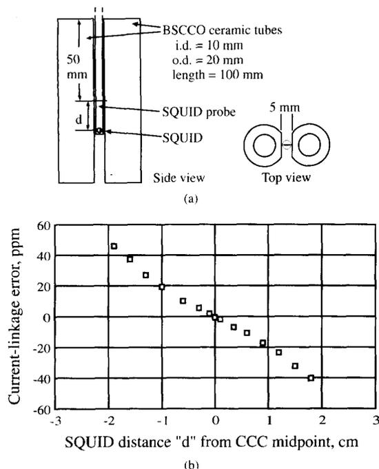
Fig. 1. (a) BSCCO tubes and a YBCO RF-SQUID in the CCC configuration, windings not shown. (b) Measurements of the current-linkage error for two windings of the BSCCC CCC as a function of the position of the SQUID.
