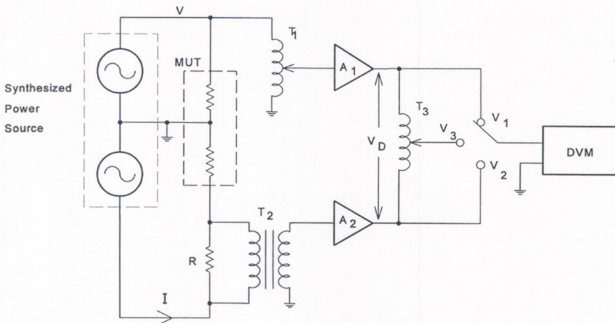
Fig. 1. Simplified diagram of the wattmeter based on rms voltage measurements.
