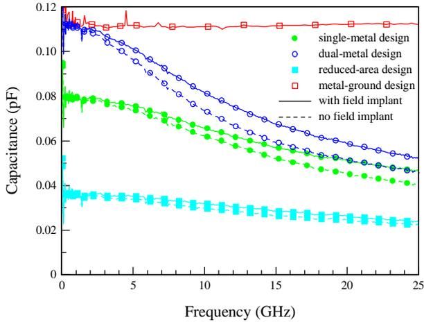
Fig. 2. Pad capacitance.
