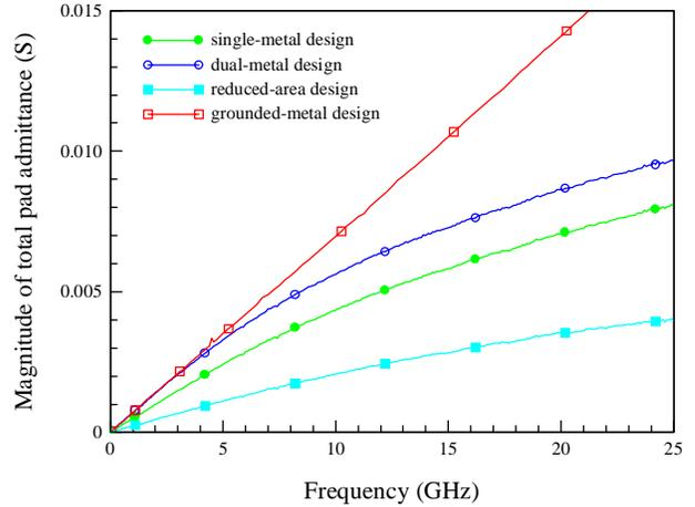
Fig. 4. Total pad admittance (with field implant).
