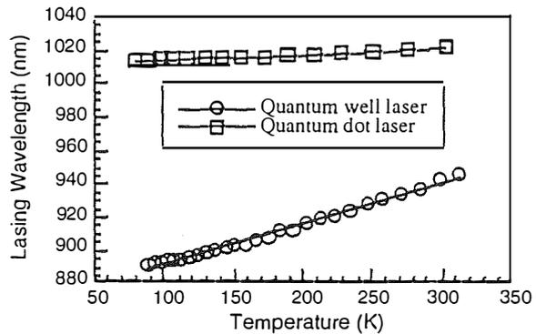
Figure 3 Lasing wavelength versus temperature for QD and QW lasers. The solid lines are linear curve fits to the data.
