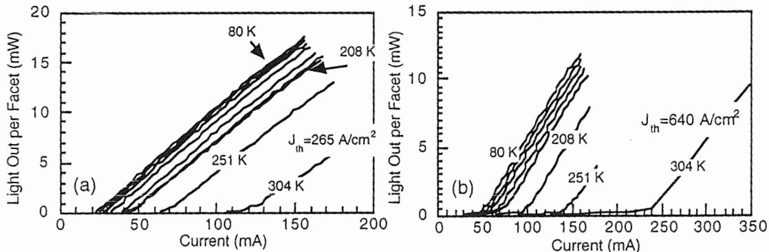
Figure 1 (a) L-I curves from an 800  $\mu\text{m}$  long QW laser at various temperatures, and (b) L-I curves from an 800  $\mu\text{m}$  long QD laser at various temperatures.
