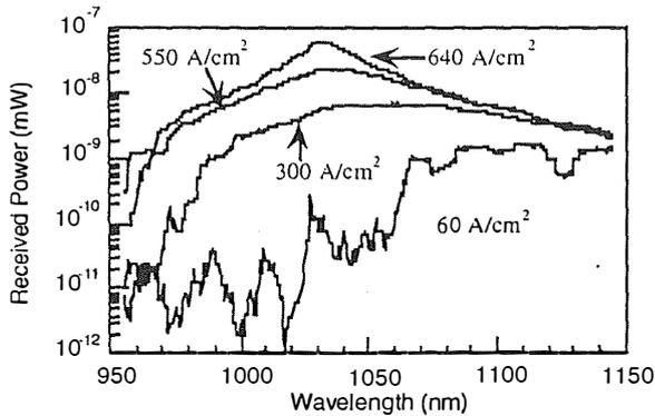
Figure 2 Subthreshold EL from the QDL at various current densities. The ground state emission is at 1150 nm.
