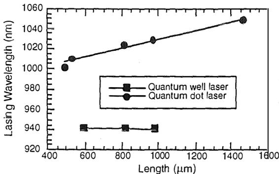
Figure 4 The quantum dot lasing wavelength changes dramatically as the laser length changes. The quantum well lasing wavelength barely changes.
