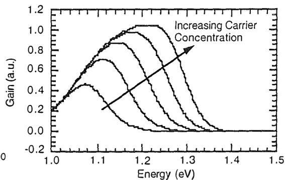
Figure 5 Gain versus energy for a quantum dot DOS that includes the energetic distribution of the discrete states due to size fluctuations in the quantum dots.
