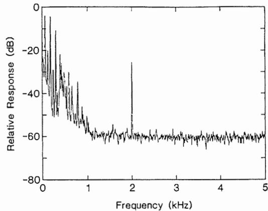
Fig. 4. Sensor output spectrum recorded while a 1.1-nT test signal is applied to the head at 2 kHz.
