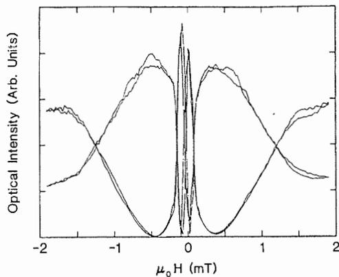
Fig. 3. Response function curves for the head in the maximum sensitivity ( $d = 0$ ) configuration and maximum field  $|\mu_0 H_{\max}| = 1.9$  mT.
