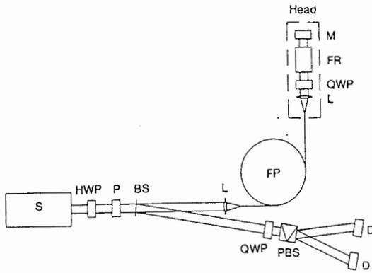
Fig. 1. Polarization-rotated reflection sensor system: S, source (laser or light-emitting diode); HWP, half-wave plate; P, polarizer; BS, beam splitter; L, lenses; FP, high-birefringence fiber pigtail; QWP, quarter-wave plates; FR, Faraday rotator; M, mirror; PBS, Wollaston polarizing beam splitter; D, detectors.
