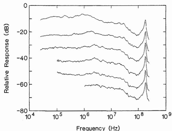
Fig. 5. Frequency response of the sensor head. The field amplitude was decremented in steps of 10 dB between runs. The top curve was recorded at a field strength of 6.8  $\mu\text{T}$  (rms).
