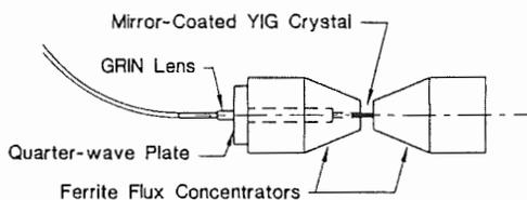
Fig. 2. Sensor head. Packaging is not shown.
