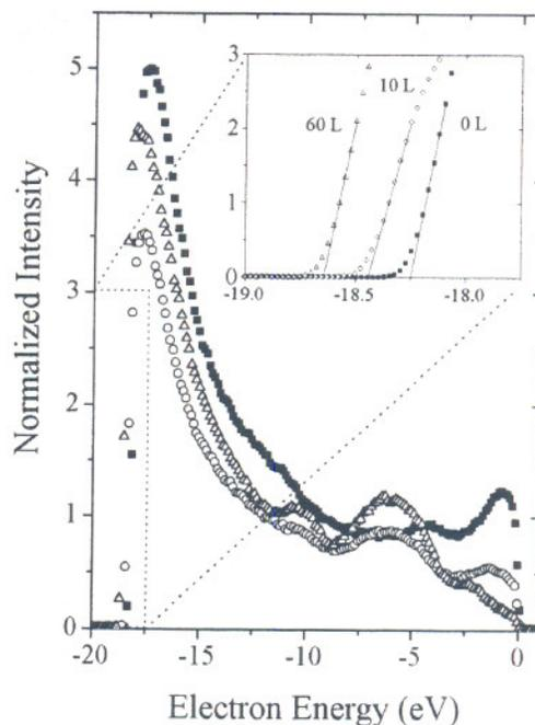
FIG. 1. Photoelectron spectra for a stainless steel surface are shown for a clean surface ( $\blacksquare$ ) and surfaces exposed to 10 L ( $\circ$ ) and 60 L ( $\triangle$ ) of oxygen. The inset clearly illustrates the change (decrease) in the work function as oxygen accumulates on the surface. The zero of the energy scale refers to a photoelectron from the top of the conduction band.
