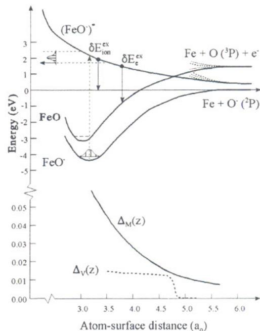
FIG. 5. Schematic diagram of the molecular states for the interaction of O and  $O^-$  with Fe as a function of distance from the surface. Also shown are the decay widths used to describe the two electron decay channels. The  $FeO$  and  $FeO^-$  ground states are representative of isolated molecular curves.
