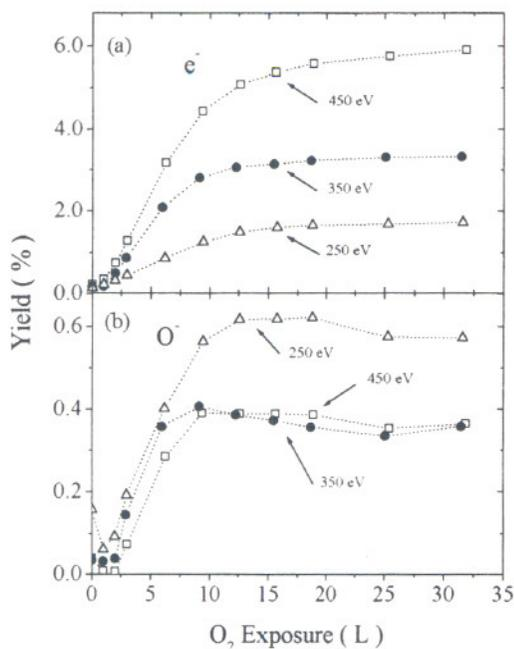
FIG. 2. (a) Absolute electron yields for  $Na^+$  impacting stainless steel at 250 eV ( $\Delta$ ), 350 eV ( $\bullet$ ), and 450 eV ( $\square$ ) as a function of oxygen exposure. (b) Absolute  $O^-$  yields for the same  $Na^+$  impact energies.
