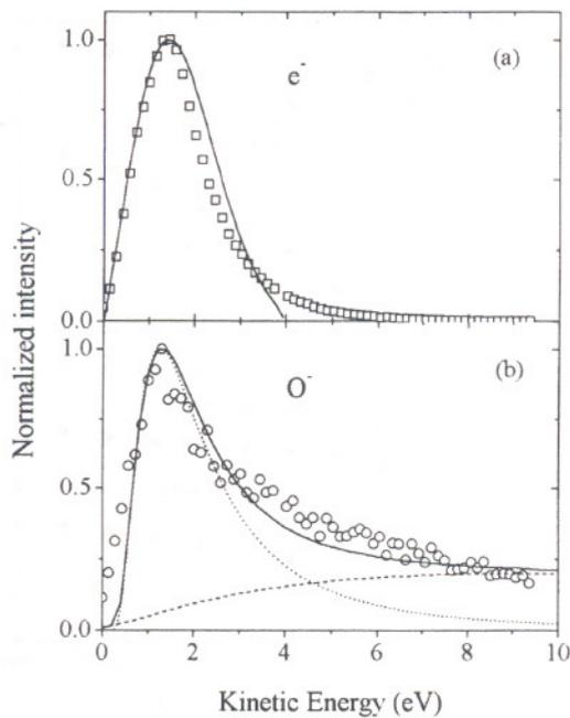
FIG. 4. (a) The electron kinetic energy distributions for a 12 L oxygen exposed stainless steel surface at an impact energy of 450 eV. The solid line is the distribution predicted by the excitation mechanism. (b) The  $O^-$  kinetic energy distribution for the same conditions. The dotted line is the distribution predicted by the excitation mechanism and the dashed line is the distribution predicted by the modified collision cascade. The solid line represents the sum of the two distributions.
