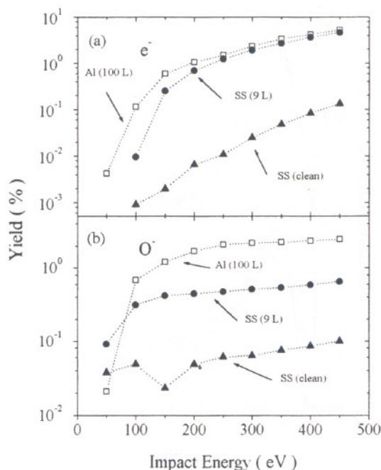
FIG. 3. (a) A comparison of the absolute electron yields for aluminum and stainless steel as a result of  $Na^+$  impact. The ( $\square$ ) are for an Al substrate exposed to 100 L of oxygen, while ( $\blacktriangle$ ) are the results for clean stainless steel surface and ( $\bullet$ ) for an exposure of 9 L. (b) A comparison of  $O^-$  yields for the same conditions.
