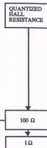
Figure 1. Measurement sequence for the comparison of the QHR and the realization of the SI ohm through the 1000\, \Omega transportable resistor.
