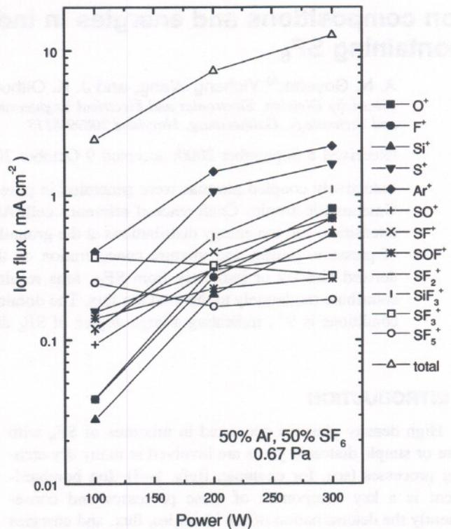
FIG. 3. Mass-resolved ion fluxes from 50%  $\text{SF}_6$ /50% Ar discharges at various powers. All discharges were sustained at 0.67 Pa (5 mTorr).
