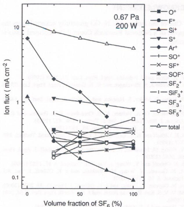
FIG. 4. Mass-analyzed ion fluxes in discharges containing SF<sub>6</sub> for various mixtures with Ar. All discharges operated at 0.67 Pa (5 mTorr) and 200 W.
