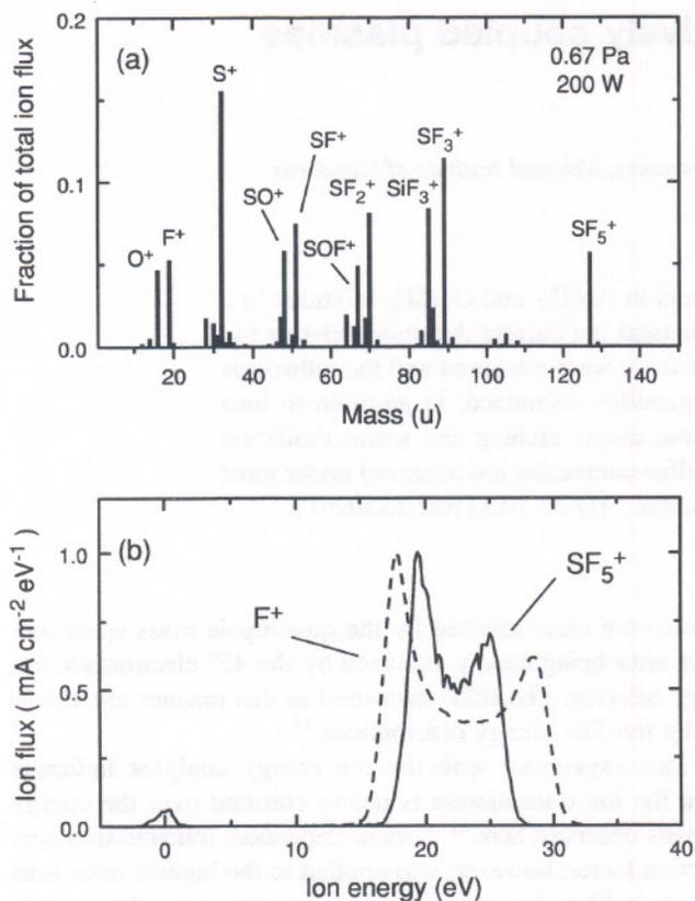
FIG. 1. (a) Mass spectrum of ions striking the grounded electrode in an inductively coupled  $\text{SF}_6$  discharge sustained at 0.67 Pa (5 mTorr) and 200 W. (b) Normalized energy distributions of  $\text{SF}_5^+$  (solid lines) and  $\text{F}^+$  (dashed lines) ions under these conditions.
