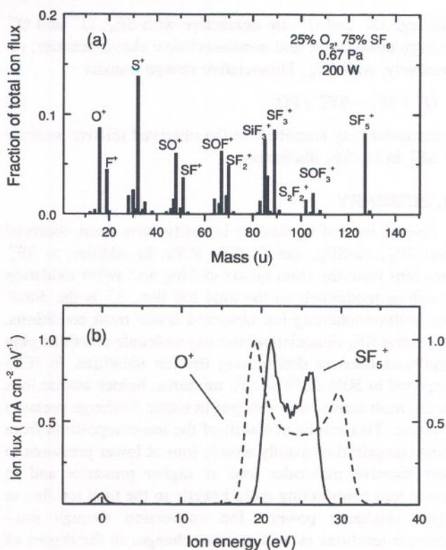
FIG. 5. (a) Mass spectrum of ions striking the grounded electrode in 75% SF<sub>6</sub>/25% O<sub>2</sub> discharge sustained at 0.67 Pa (5 mTorr) and 200 W. (b) Normalized energy distributions of SF<sub>5</sub><sup>+</sup> (solid lines) and O<sup>+</sup> (dashed lines) ions under these conditions.
