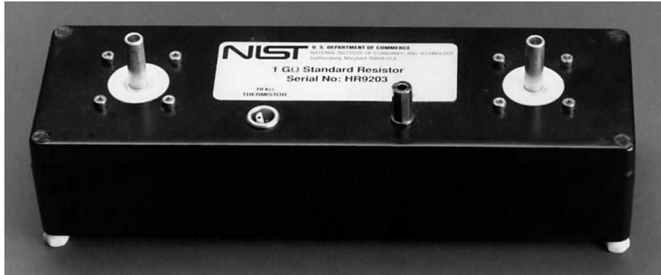
Fig. 2. Completed 1 GΩ standard resistor with coaxial terminals mounted on circular PTFE plates.
