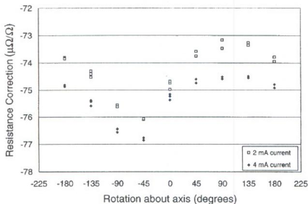
Fig. 4. Resistance correction from the nominal value of 1000  $\Omega$  for resistor SFA. The graph shows changes in resistance for two current levels as a function of the placement of the resistor, for rotation of the resistor case about the long axis. The changes are related to reversible strain caused by bending of the resistance element.
