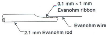
Fig. 2. Spot-welded Evanohm wire as used in the new coaxial resistors.
