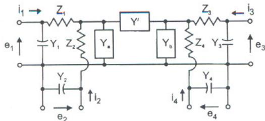
Fig. 1. Four-terminal-pair coaxial resistor represented by an equivalent circuit, with  $Y'$  as the series admittance of the main resistance element,  $Y_a$  and  $Y_b$  as the shunt admittances of the coaxial elements, and other impedances and admittances of the leads and connections as shown.
