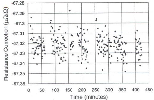
Fig. 3. Sequence of data showing the resistance correction from the nominal value of 100  $\Omega$  for coaxial resistor SCA. The random uncertainty of each data point is about 0.01  $\mu\Omega/\Omega$ .
