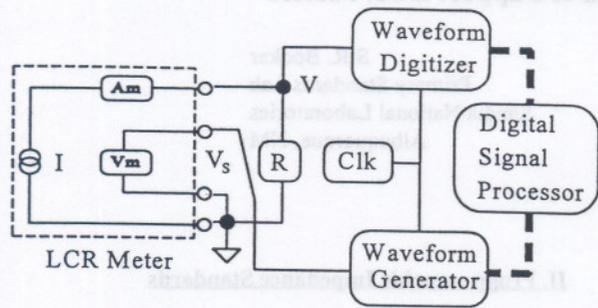
Fig. 1. Digitally synthesized impedance generator that samples the LCR meter test current, modifies it digitally, and reconstructs a voltage waveform using a waveform generator. Heavy dashed lines represent a data bus.
