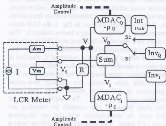
Fig. 2. Analog impedance generator that uses MDACs and an integrator to generate in-phase and quadrature components.
