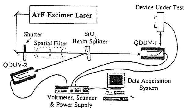
**Figure 1.** NIST UV measurement system for 193 nm laser power and energy measurements. QDUV-1 and QDUV-2 are the primary standard calorimeters. A 2° wedged, fused silica (SiO<sub>2</sub>) beamsplitter is used for monitoring the power and providing attenuation.
