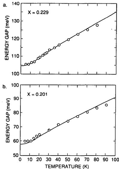
Figure 1. a.) Energy gap of sample with  $x = 0.229$  as a function of temperature. The fit by our new relation with  $x = 0.2285$  is the solid line. b.) Energy gap of sample with  $x = 0.201$  as a function of temperature. The fit by our new relation is the solid line.
