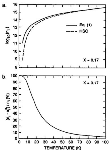
Figure 2. a.) Logarithm of the intrinsic carrier density,  $n_i$ , ( $\text{cm}^{-3}$ ) as a function of temperature for  $x = 0.17$ . The solid line is with our new relation and the dotted line is with the HSC relation. b.) The percentage difference between  $n_i$  from our new relation and  $n_i^H$  from the HSC relation, relative to our new relation.
