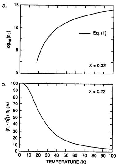
Figure 3. a.) Logarithm of the intrinsic carrier density,  $n_i$ , ( $\text{cm}^{-3}$ ) as a function of temperature for  $x = 0.22$ . The solid line is with our new relation. b.) The percentage difference between  $n_i$  from our new relation and  $n_i^H$  from the HSC relation, relative to our new relation.
