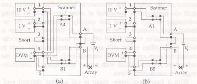
Fig. 2. A simplified internal wiring schematic illustrating two different switch configurations. (a) Selections A4 and B1. (b) Selections A1 and B5. To maintain the DVM polarity of the first circuit but interchange the array and 10-V source, the reverse DVM of channel 5 must be used.
