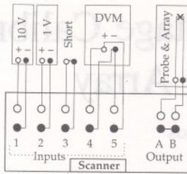
Fig. 1. An illustration of the array system connections at the back panel the scanner. Inputs 1 and 2 are Zener references, 3 is short, and 4 and 5 are DVM connections reversed relative to each other. The array within its cryoprobe circuit is at the output terminals; the common output terminals are shorted.
