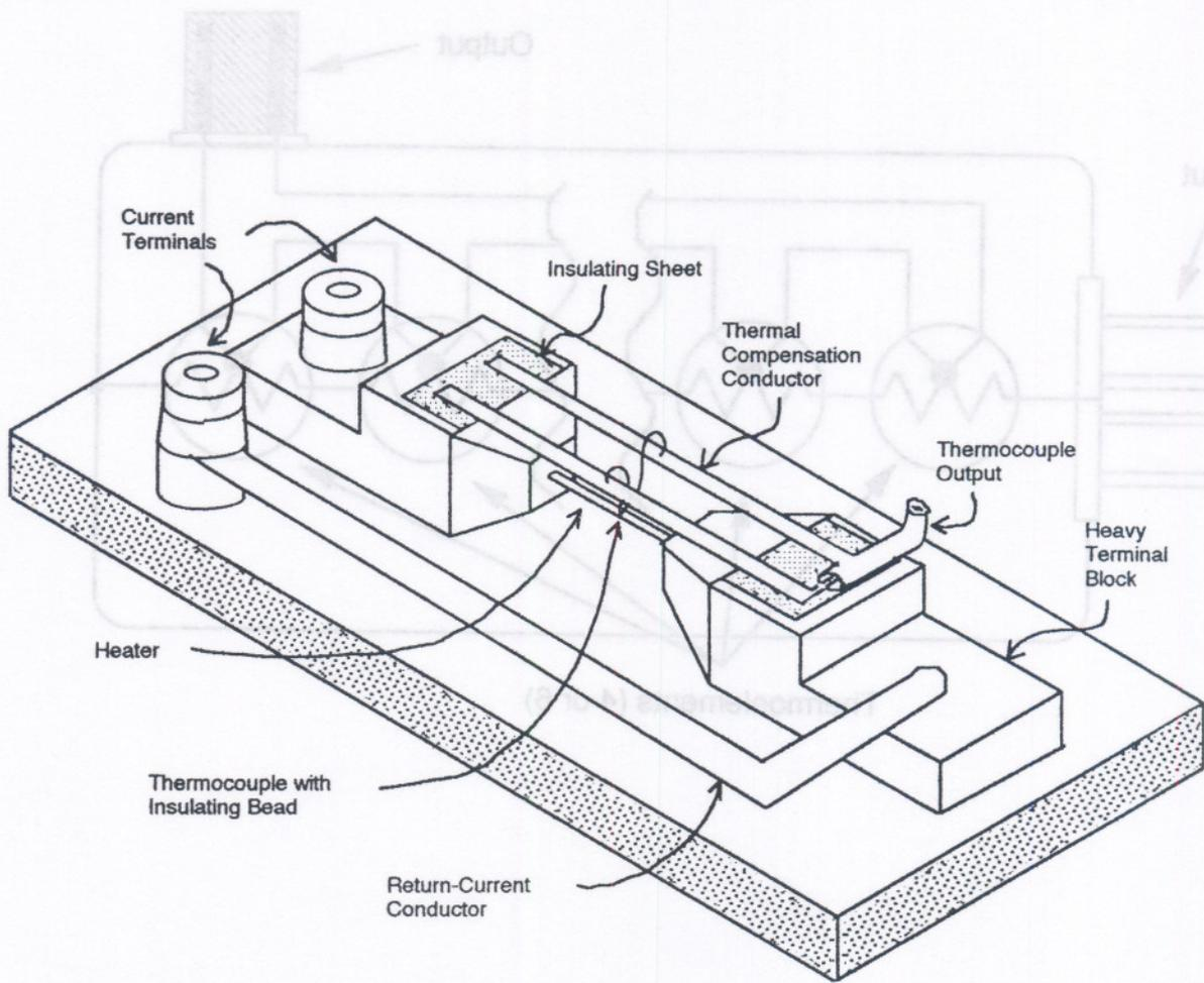
Figure 1. Diagram of low-frequency thermal converter module, consisting of either four (or six) or six (or four) thermal elements with their inputs and outputs connected in series.
