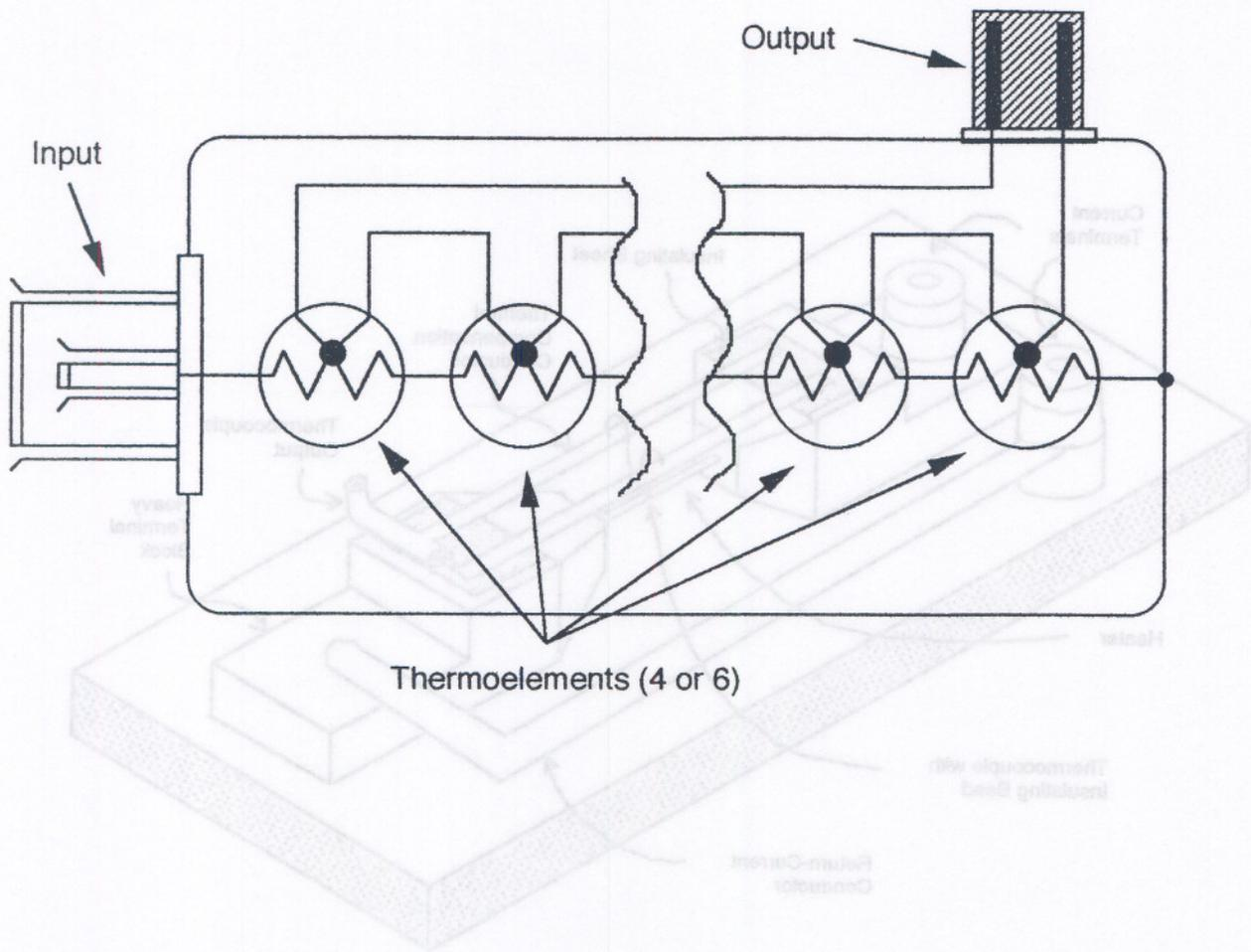
Figure 1. Diagram of low-frequency thermal converter module, consisting of either four (for Fe) or six (for Ru) thermal elements with their inputs and outputs connected in series.
