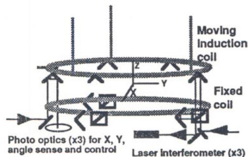
Figure 1. Coil schematic showing interferometer and alignment optics.
