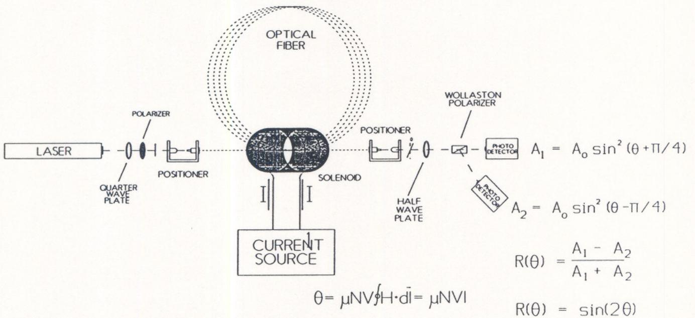
Figure 2 – Example of a system in which the Faraday effect is used to measure current.
