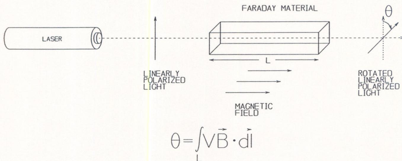
Figure 1 - The Faraday effect. When linearly polarized light from a laser passes through an optically active material of length  $L$  parallel to the direction of an applied magnetic field, the plane of polarization of the light will be rotated by an angle  $\theta$  as shown.
