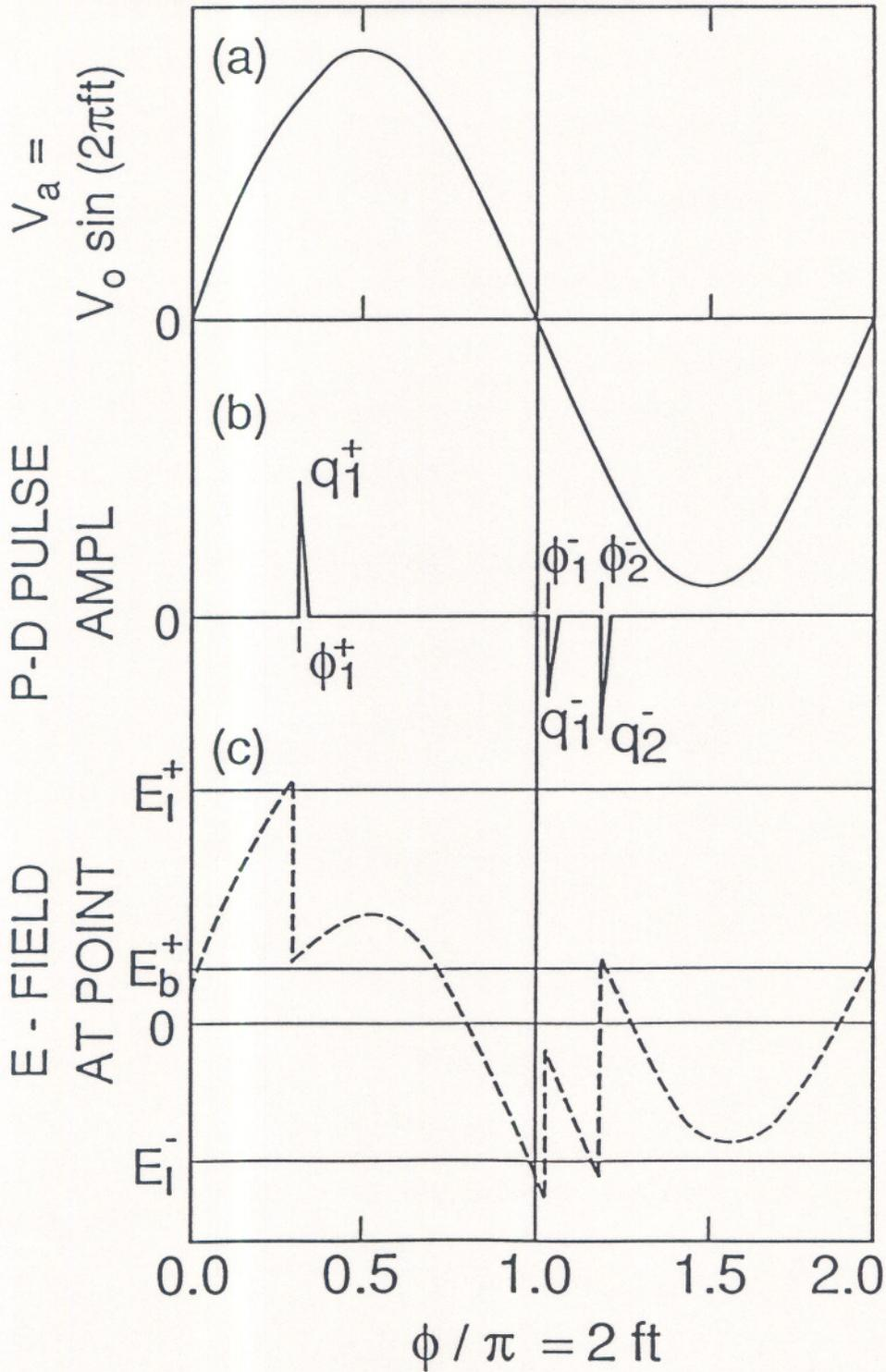
Figure 3 - Diagrammatic representation of an ac-generated PD process. Shown is the applied voltage ( $V_a$ ), the local electric field strength at the discharge site ( $E$ ), and the amplitudes ( $q_i^\pm$ ) and phases ( $\phi_i^\pm$ ) of the individual PD pulses. Onset levels ( $E_i^\pm$ ) and a possible constant bias level ( $E_b^+$ ) are also shown.
