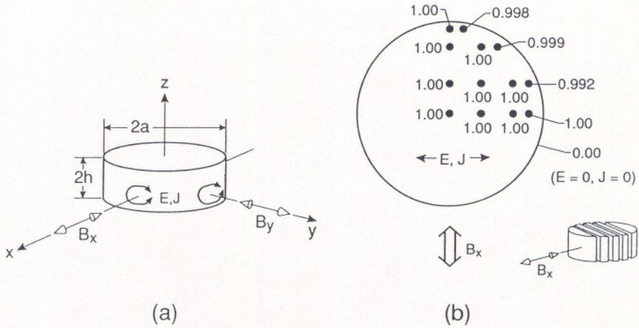
Fig. 1. Experimental configuration for in vitro studies: (a) Components of magnetic field applied parallel to x- and y-axes; (b) Normalized induced current density distribution along bottom (or top) surface of culture medium for uniform magnetic field parallel to x-axis for  $2a = 6$  cm and  $2h = 0.2$  cm.
