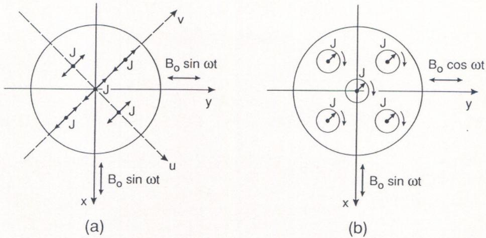
Fig. 2. (a) Induced current sheet oscillates along fixed direction for linearly polarized magnetic field. (b) Induced current sheet rotates with constant magnitude for circularly polarized magnetic field.
