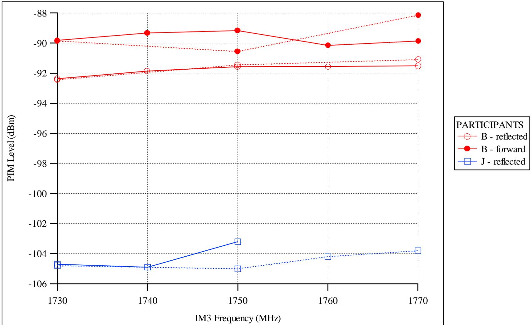
**Figure 17.** Measurements of the WHITE round-robin artifact in the DCS band.
