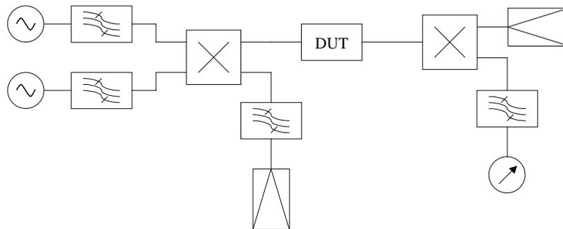
**Figure 3.** Two configurations for measuring passive intermodulation products: reflected and forward.
