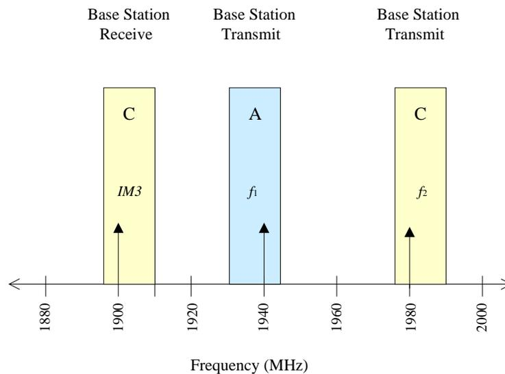
**Figure 1.** Potential third-order intermodulation in broadband PCS.
