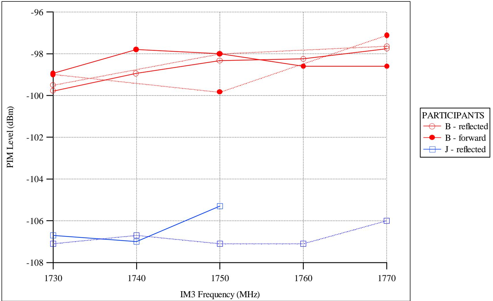
**Figure 16.** Measurements of the RED round-robin artifact in the DCS band.
