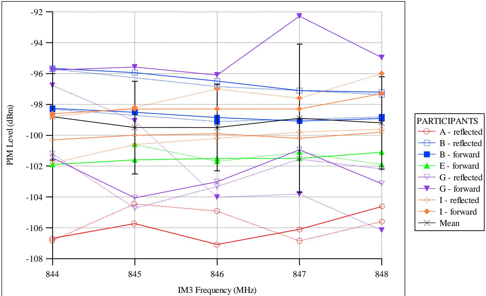
Figure 5. Measurements of the WHITE round-robin artifact in the AMPS band.
