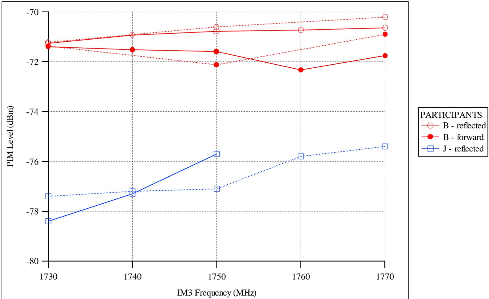
**Figure 18.** Measurements of the YELLOW round-robin artifact in the DCS band.
