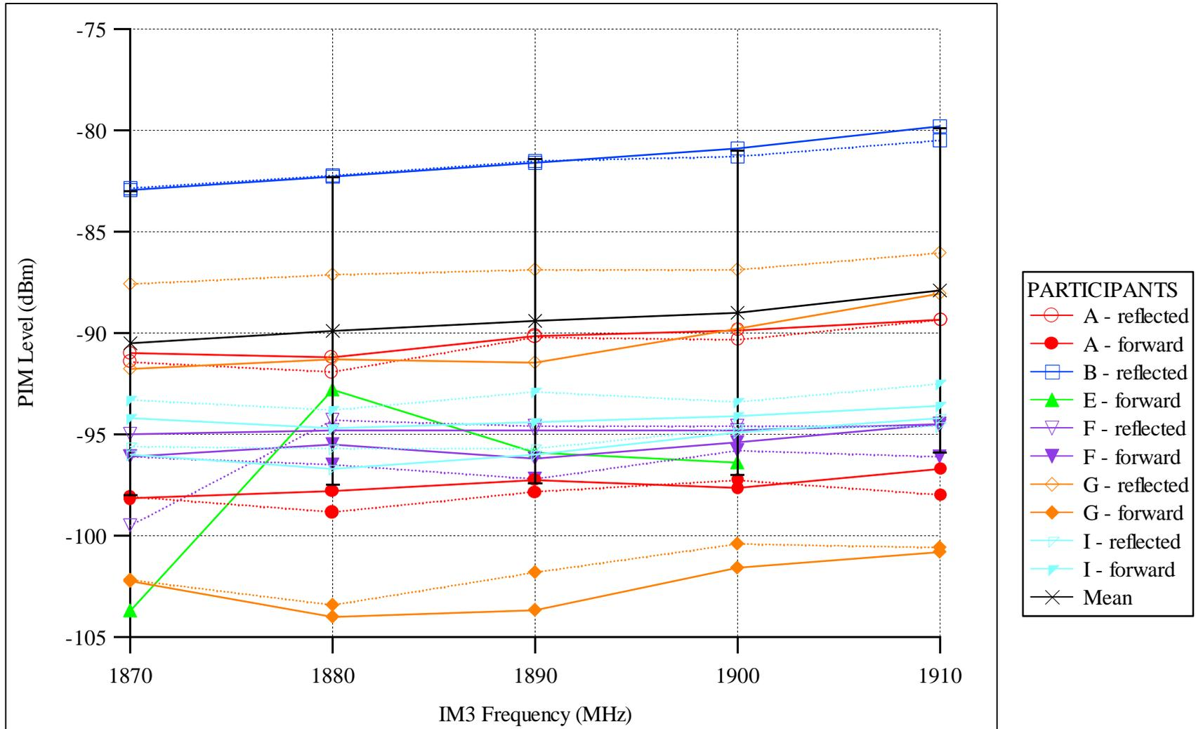
**Figure 13.** Measurements of the WHITE round-robin artifact in the PCS band.
