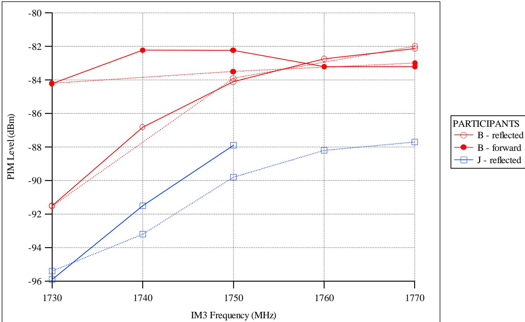
**Figure 19.** Measurements of the BLUE round-robin artifact in the DCS band.
