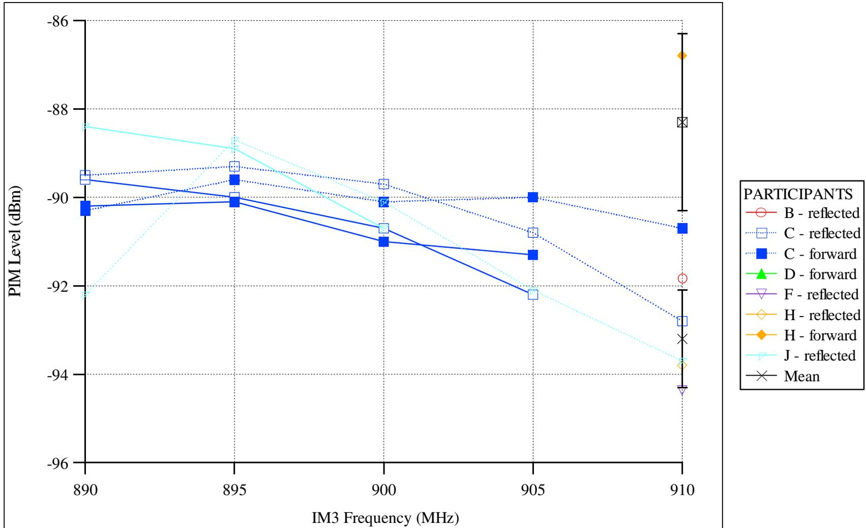
**Figure 11.** Measurements of the BLUE round-robin artifact in the GSM band, excluding participant D.
