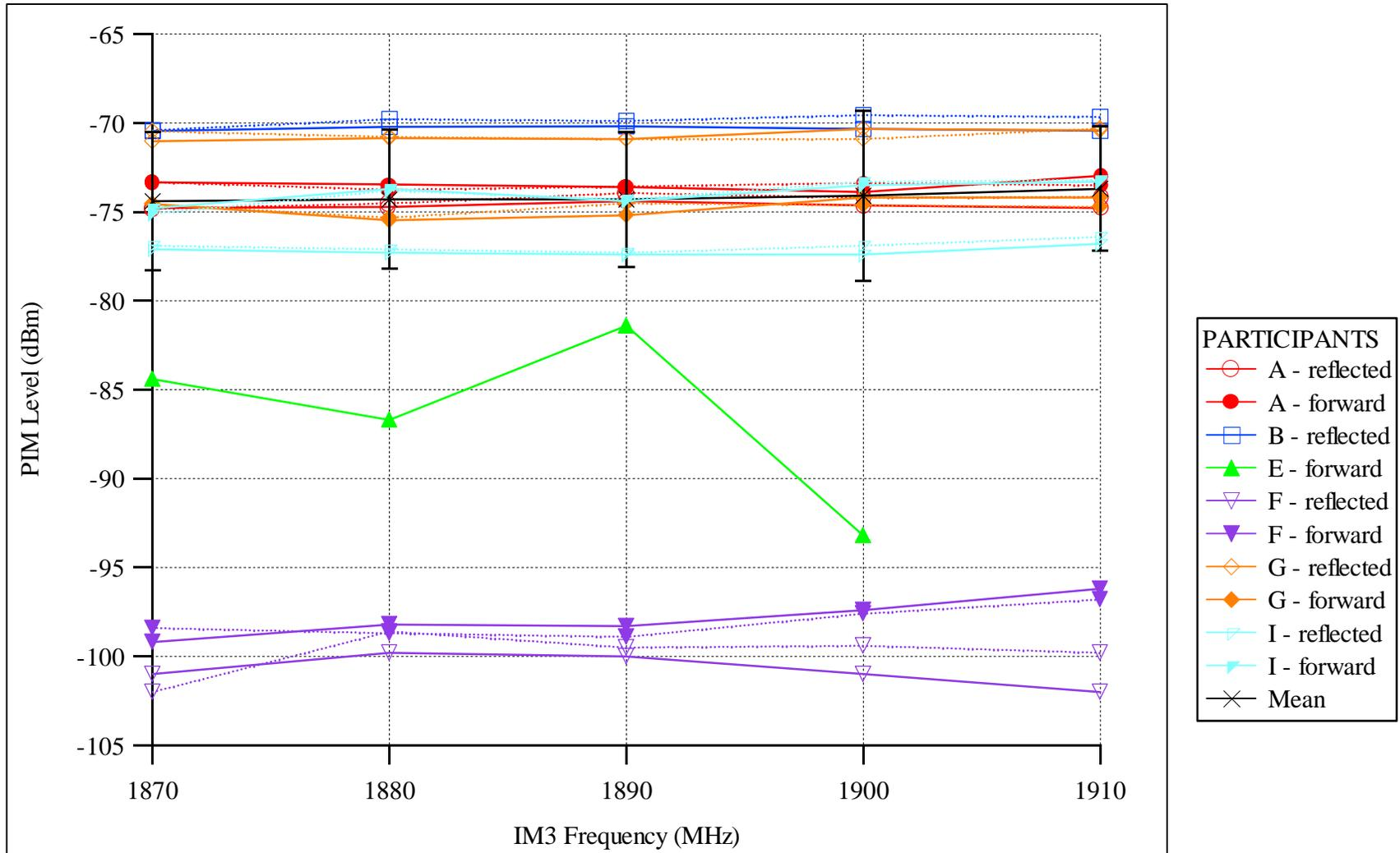
**Figure 14.** Measurements of the YELLOW round-robin artifact in the PCS band.
