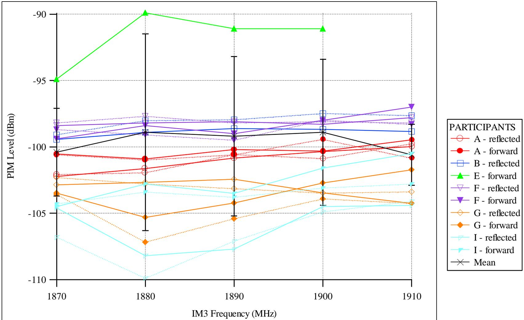
**Figure 12.** Measurements of the RED round-robin artifact in the PCS band.
