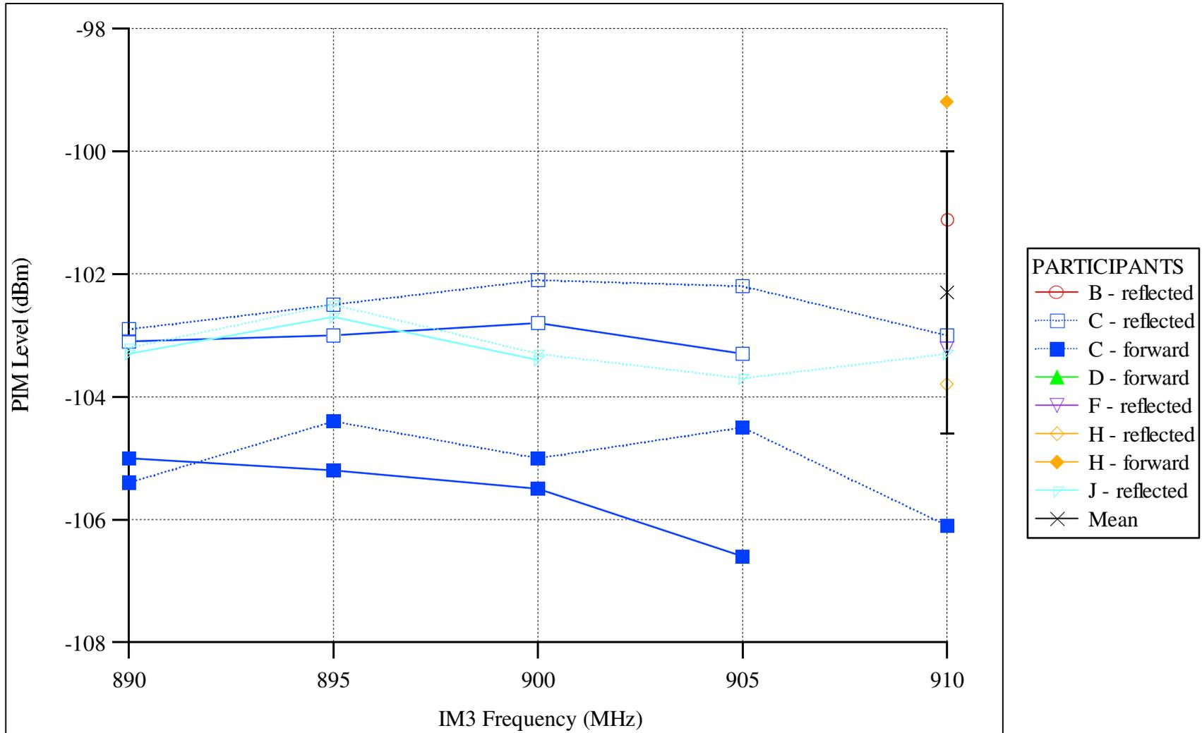
**Figure 8.** Measurements of the RED round-robin artifact in the GSM band, excluding participant D.
