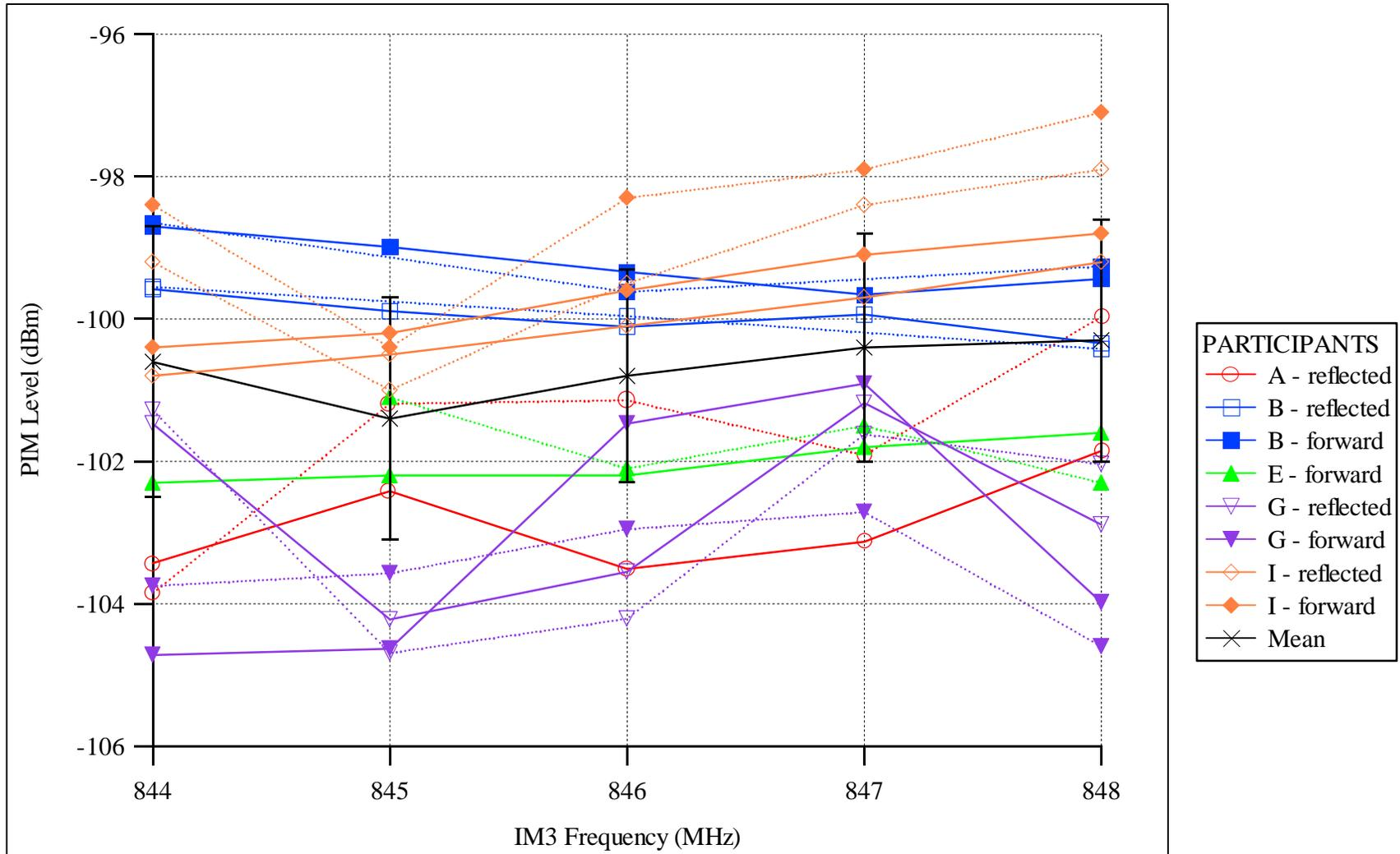
**Figure 4.** Measurements of the RED round-robin artifact in the AMPS band.
