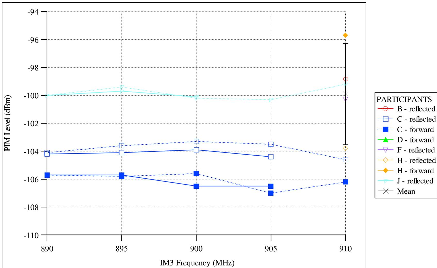
**Figure 9.** Measurements of the WHITE round-robin artifact in the GSM band, excluding participant D.
