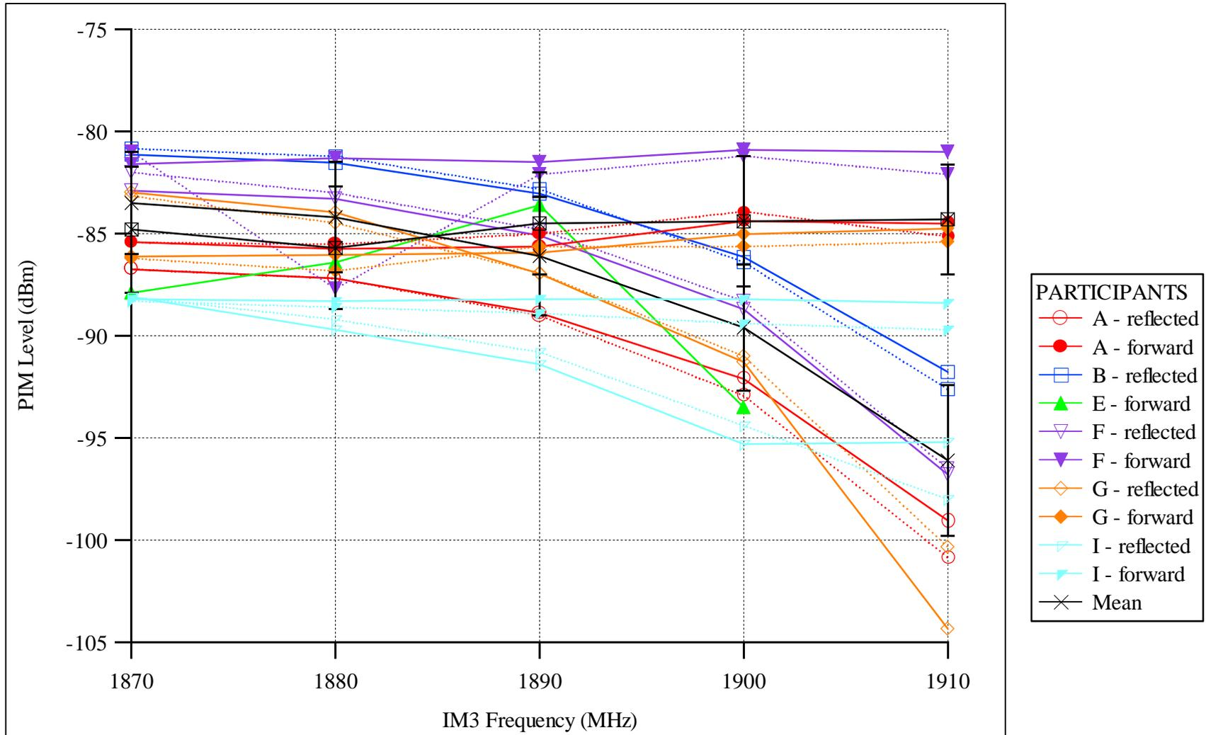
**Figure 15.** Measurements of the BLUE round-robin artifact in the PCS band.
