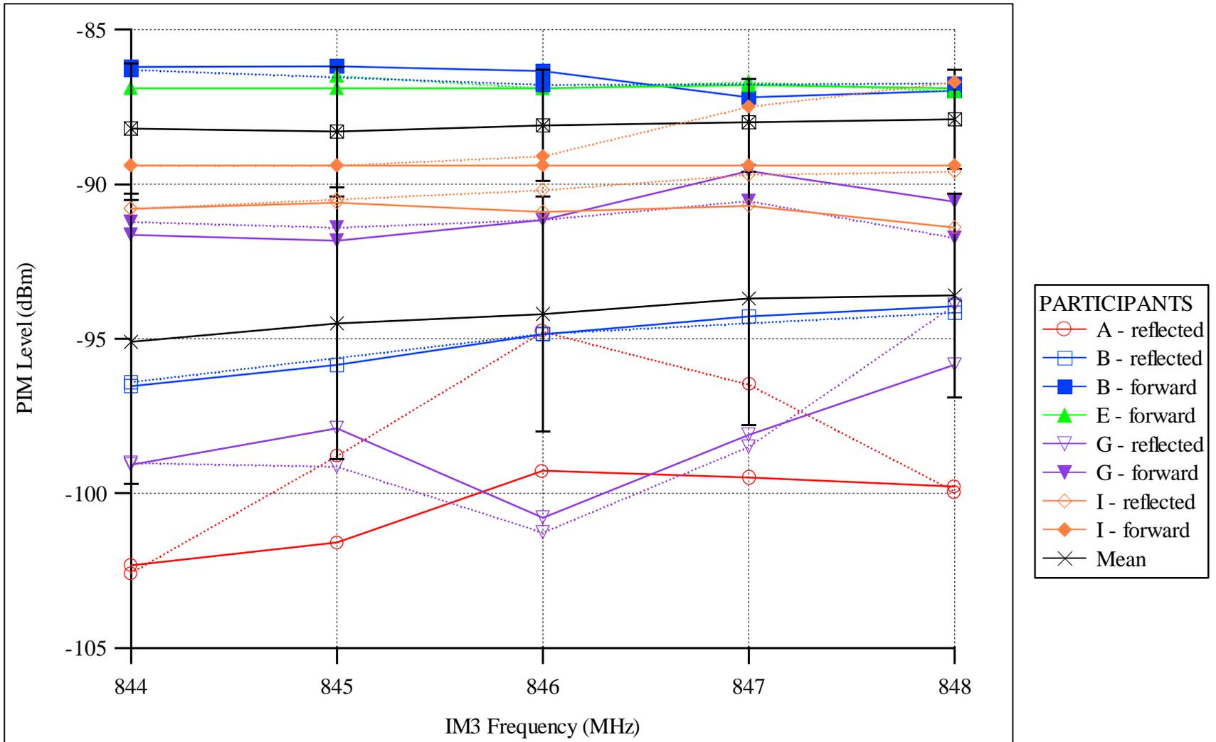
**Figure 7.** Measurements of the BLUE round-robin artifact in the AMPS band.
