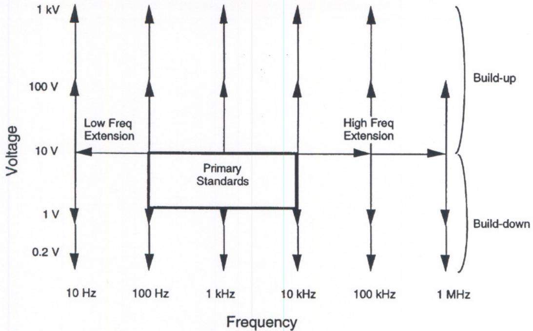
Fig. 1. Diagram of the primary standards, high and low frequency extension paths and build-up and build-down paths used to characterize standards over entire parameter space.
