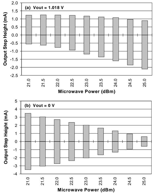
Fig. 4. Josephson array output step height vs. microwave power for (a)  $V_{out} = 1.018$  V [all cells *on*], and (b)  $V_{out} = 0$  V [all cells *off*].
