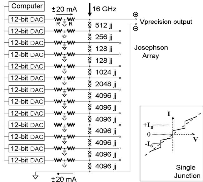
Fig. 1. Bias schematic of the 1 Volt programmable JVS.
