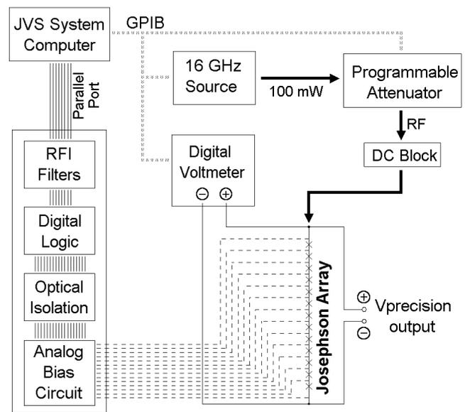
Fig. 3. Block diagram of the 1 Volt programmable JVS.
