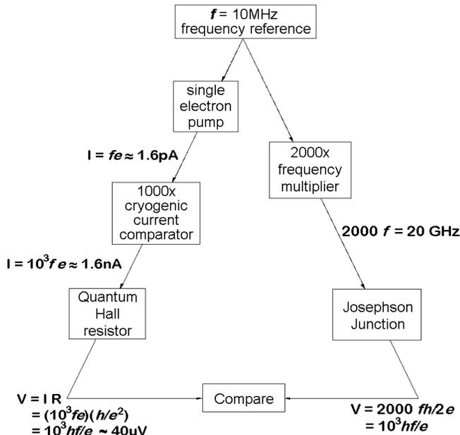
Fig. 8. Block diagram of the metrology triangle experiment.
