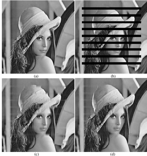
Fig. 5. Subjective comparison of different algorithms for the image "Lena". (a) The original image, (b) The corrupted image, (c) The reconstructed image by the bilinear interpolation, (d) The reconstructed image by the proposed algorithm
