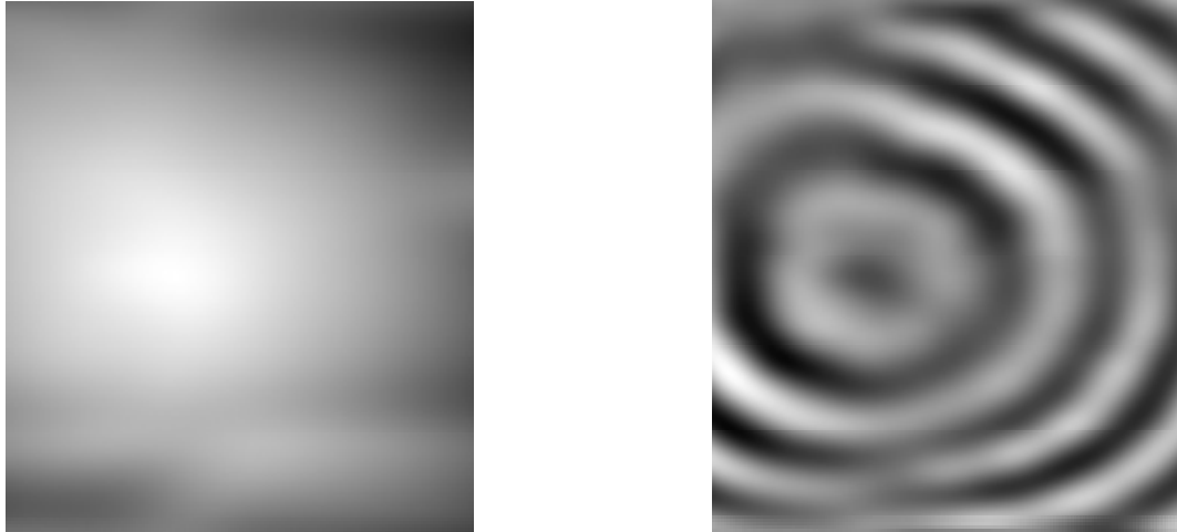
Figure 3: Non-flatness ( I_m ) and phase error ( I_p ) caused by SLM.
