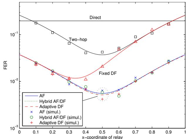
Fig. 3. FER vs. position, Rayleigh fading,  $E_b/N_0 = 7$  dB
