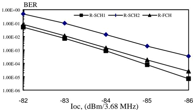
Figure 3. BER performance of the R-FCH, R-SCH1, and R-SCH2 with unequal power allocation for the supplemental channels
