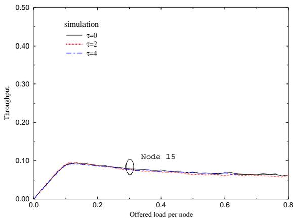
Fig. 14. Throughput of UN-guaranteed node for different  $\tau=0, 2$ , and 4.
