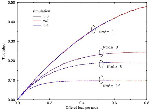
Fig. 13. Throughput of guaranteed nodes for different  $\tau=0, 2$ , and 4.
