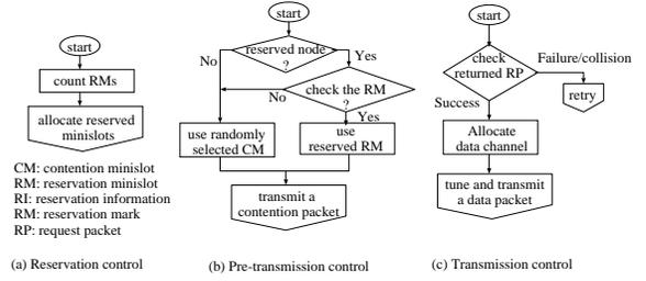
Fig. 6. Flow diagrams of the proposed protocol.
