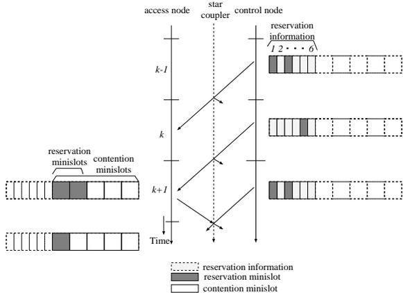
Fig. 7. An example of reservation control procedure.
