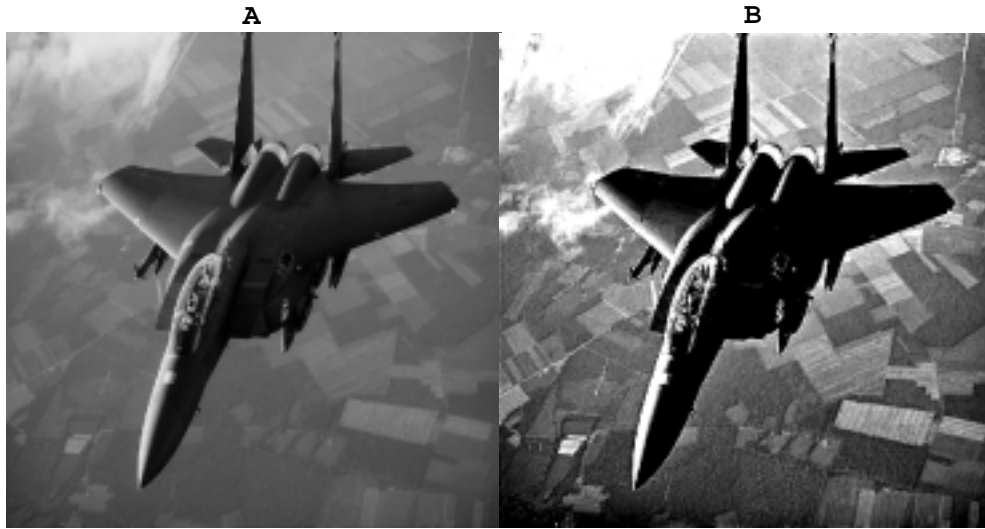
FIG. 12. Striking enhancement of terrain features in an F15 image. The APEX method with A = 3.5 on |\xi| \leq 250 yields \alpha = 0.856096 , \beta = 0.107289 . Using these parameters, with s = 0.01 , K = 1000 , and backwards continuation terminated at t = 0.25 , the SECB method applied to image (a) produced image (b). Condensation trails behind the aircraft in image (b) were not immediately evident in image (a).
