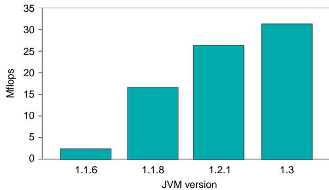
**Figure 2. Evolution of Java performance for the SciMark benchmark on a single platform: a 333-MHz Sun Ultra 10.**
