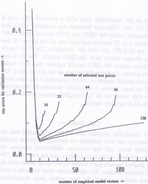
Fig. 5. Rms difference between predicted values and true values using SVD derived models and an rms measurement of 0.1.
