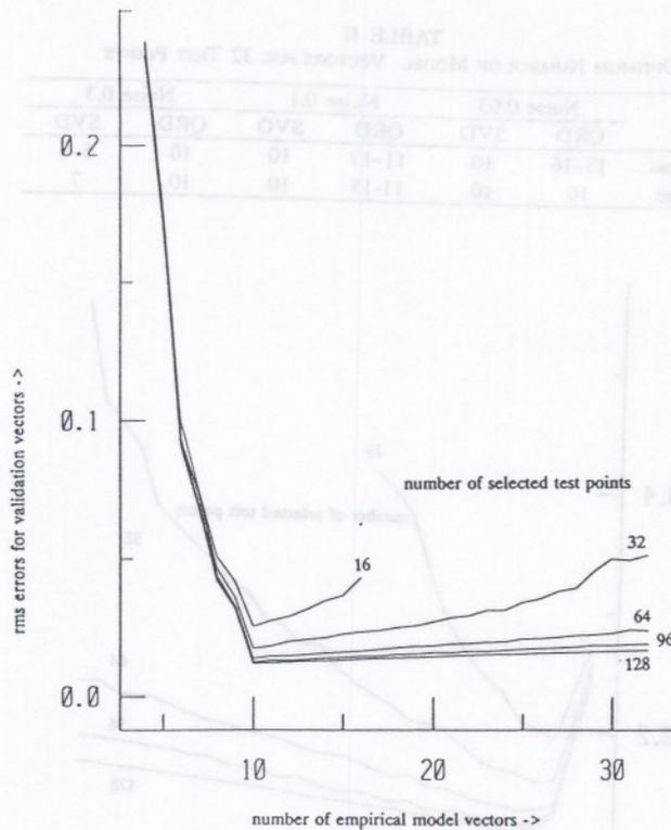
Fig. 7. Rms difference between predicted values and true values using SVD derived models and an rms measurement noise of 0.03.
