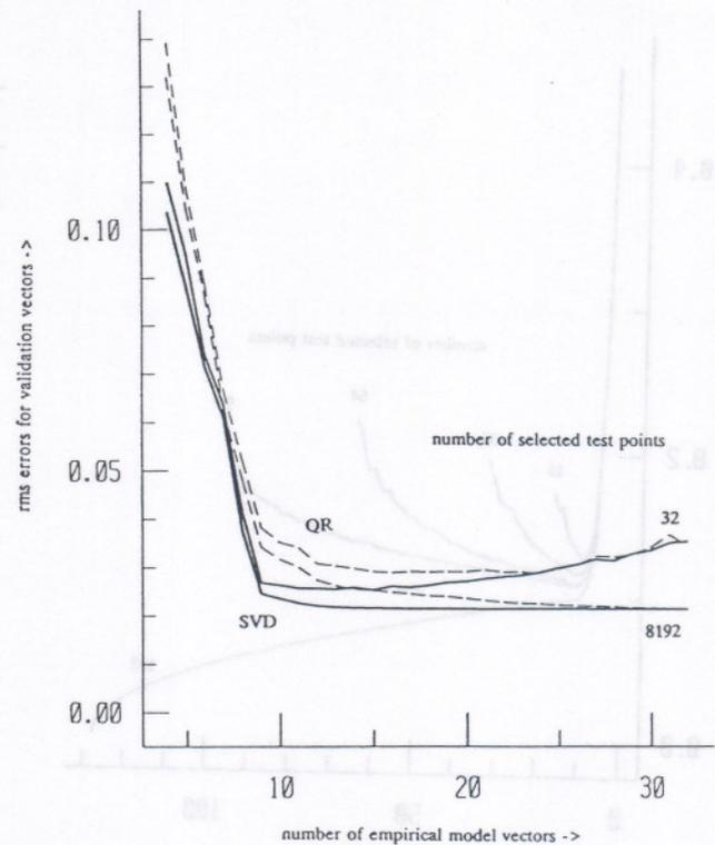
Fig. 8. Rms difference between predicted values and measured values using QRD derived models (dashed lines) and SVD derived models (solid lines) for data from 13-bit A/D converters with an rms measurement noise of about 0.021.
