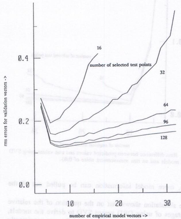
Fig. 6. Rms difference between predicted values and true values using SVD derived models and an rms measurement noise of 0.3.
