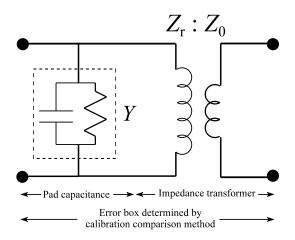
Fig. 2. The equivalent-circuit model for the contact pads and impedance transformer used in the calibration-comparison method for measuring characteristic impedance.
