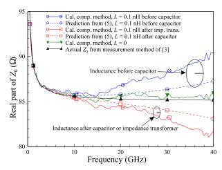
Fig. 3. Actual measurement errors compared to prediction from (5).
