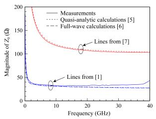
Fig. 1. Comparisons of the calibration-comparison method for measuring characteristic impedance to calculation.
