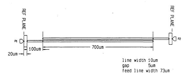
FIGURE 2. Layout of 35 GHz DC Block
