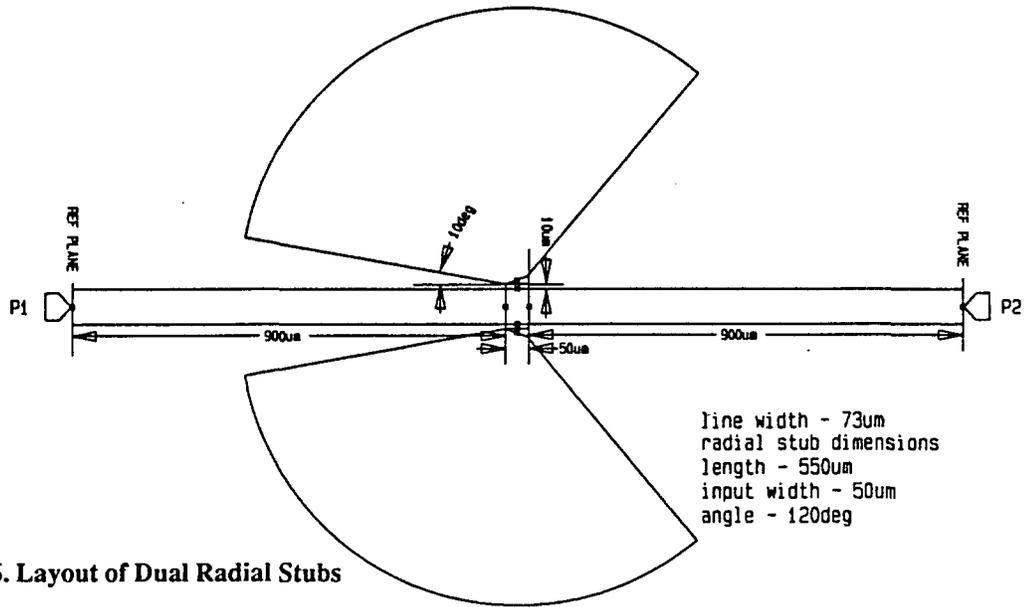
FIGURE 6. Layout of Dual Radial Stubs
