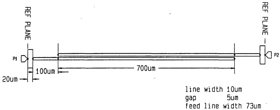
**FIGURE 2. Layout of 35 GHz DC Block**
