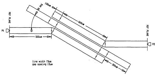
FIGURE 4. Layout of the 35 GHz Band Pass Filter
