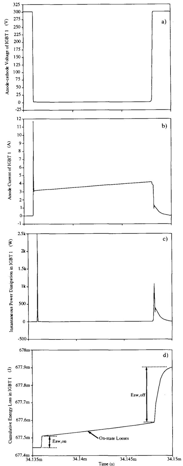
Fig. 8. One switching cycle from the 20.1 kHz simulation for the a) anode-cathode voltage, b) anode current, c) instantaneous dissipated power, and d) the cumulative dissipated energy for IGBT 1.
