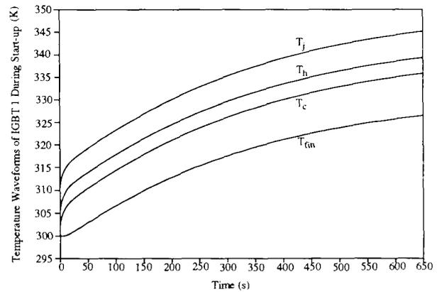
Fig. 9. Simulated thermal response at start-up for the average power dissipated in IGBT 1 indicating the temperature at the chip-package interface, the package-heat sink interface, and the heat sink fin.
