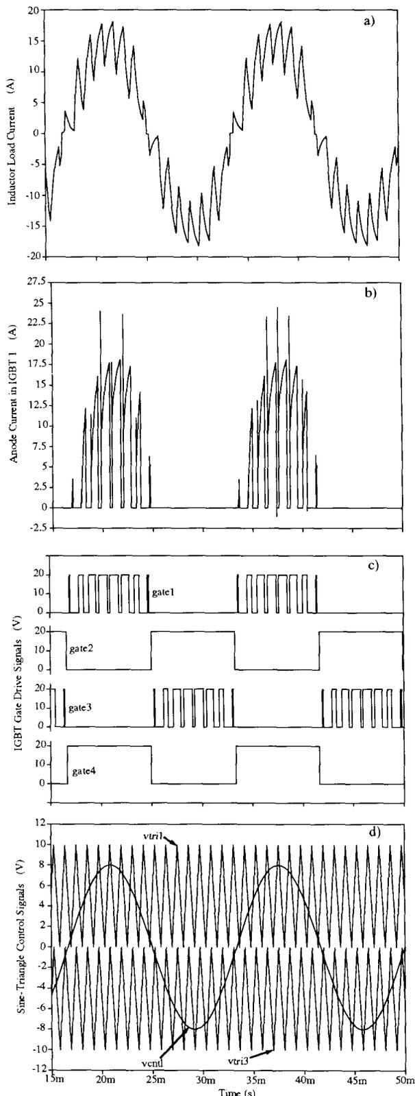
Fig. 6. Simulations of electro-thermal network of Fig. 5 for 900 Hz switching where the following curves are shown: a) motor load current, b) IGBT 1 anode current, c) logic input signals to the IGBT gate drivers, and d) the sine-triangle control signals.
