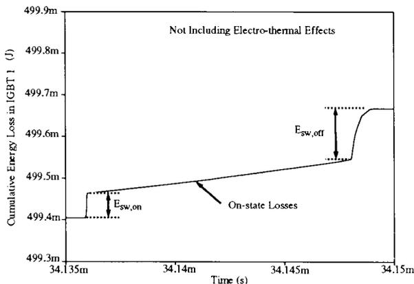
Fig. 10. Simulated energy loss neglecting the device self-heating (i.e., IGBT temperature is constant at 300 K) for the same time interval as in Fig. 8d.
