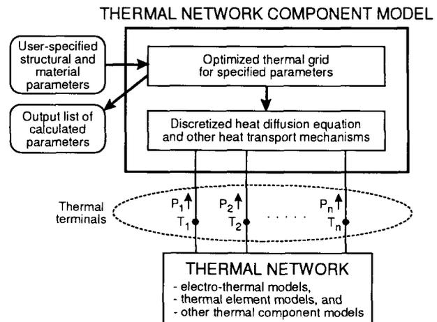
Fig. 4. Diagram of the structure of the thermal component models.
