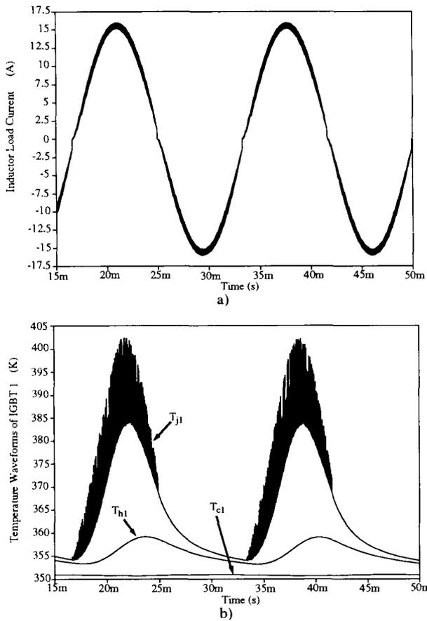
Fig. 7. Simulations of Fig. 5 with a switching frequency of 20 kHz where a) is the load current and b) is the temperature waveforms at the silicon chip surface ( $T_j$ ), the chip-package interface ( $T_h$ ), and the package-heat sink interface ( $T_c$ ) for IGBT 1.
