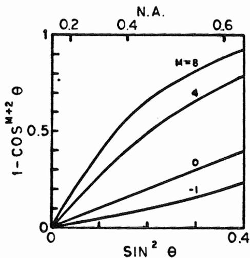
Figure 1. A function useful for describing non-Lambertian sources.
