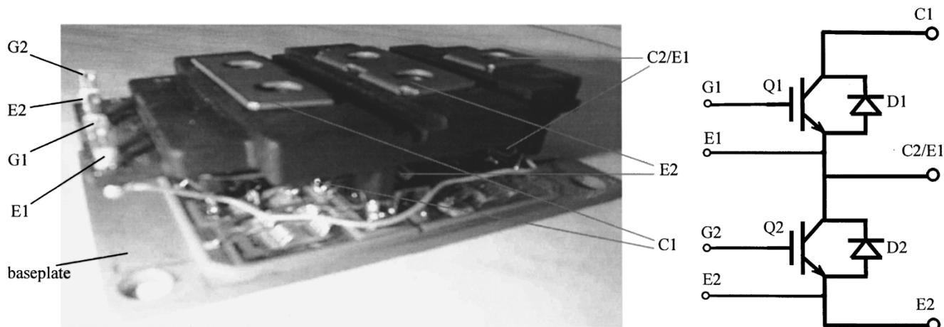
Fig. 4. A 600-V/400-A half-bridge IGBT module and its equivalent circuit diagram.
