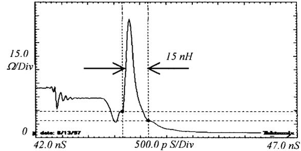
Fig. 17.  $Z$  profile of the capacitor interconnect.
