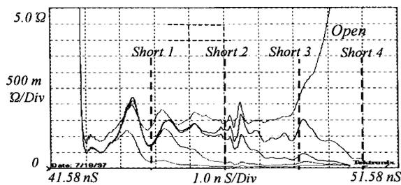
Fig. 15.  $Z$  profiles of the busbar with different shorts.
