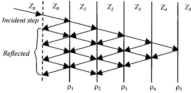
Fig. 1. Incidental step signal and its reflected responses.
