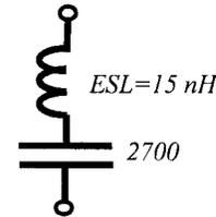
Fig. 18. Leakage inductance of the capacitor.
