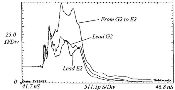
Fig. 11.  $Z$  profiles measured on gate leads of  $Q2$ .
