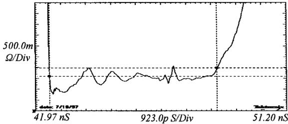
Fig. 14.  $Z$  profile of the busbar with open end.
