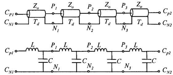
Fig. 16. Equivalent models of the busbar.
