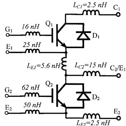
Fig. 12. Interconnect inductance of the IGBT module.
