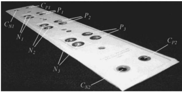
Fig. 13. The custom-designed busbar tested in experiment.
