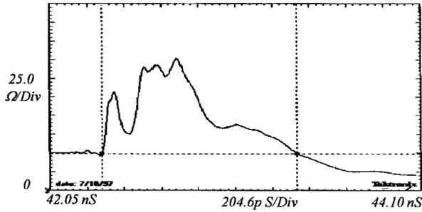
Fig. 8.  $Z$  profile of gate lead from  $G1$  to  $E1$ .
