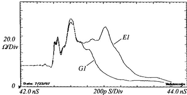
Fig. 9. Comparison of  $Z$  profiles: lead  $G1$  versus  $E1$  with respect to the base plate.
