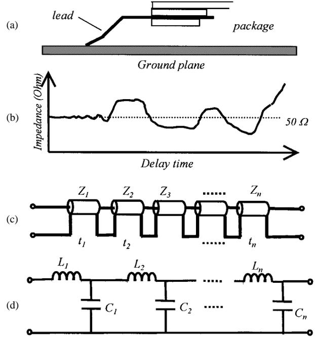
Fig. 2. A lead can be viewed as transmission line segments and modeled as  $L$ - $C$  sections of varying impedance.
