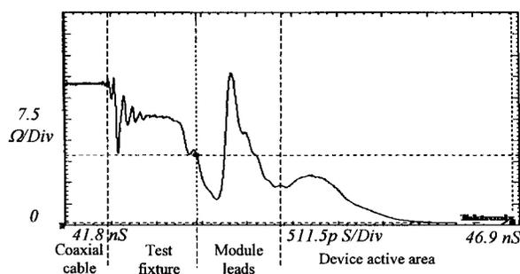
Fig. 5.  $Z$  profile of interconnect from  $E2$  to  $C2/E1$ .
