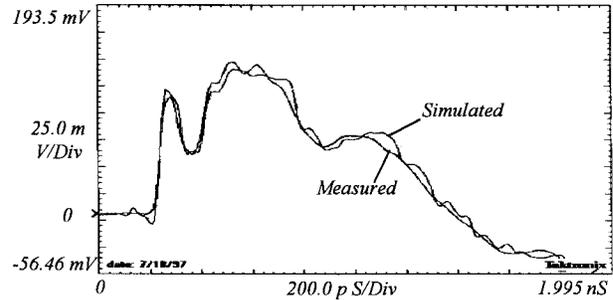
Fig. 10. Simulated versus measured TDR responses from  $G1$  to  $E1$ .
