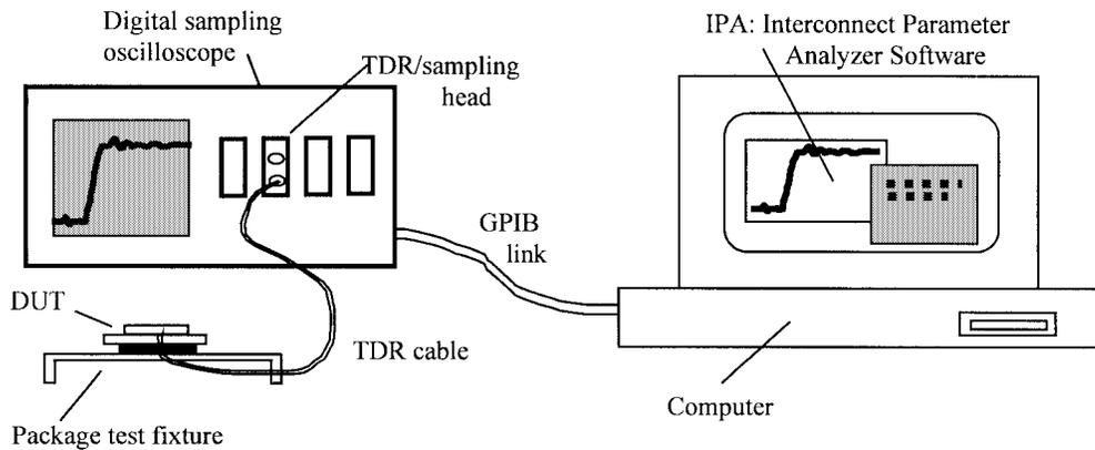
Fig. 3. Instrumentation setup of Tektronix TDR system.
