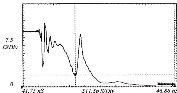
Fig. 6.  $Z$  profile of interconnect from  $C1$  to  $E2$ .
