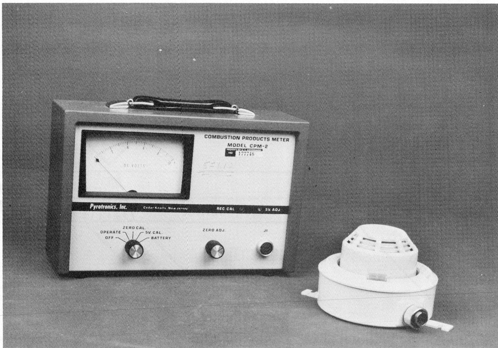
Figure 15. The Cerberus measuring ionization chamber
