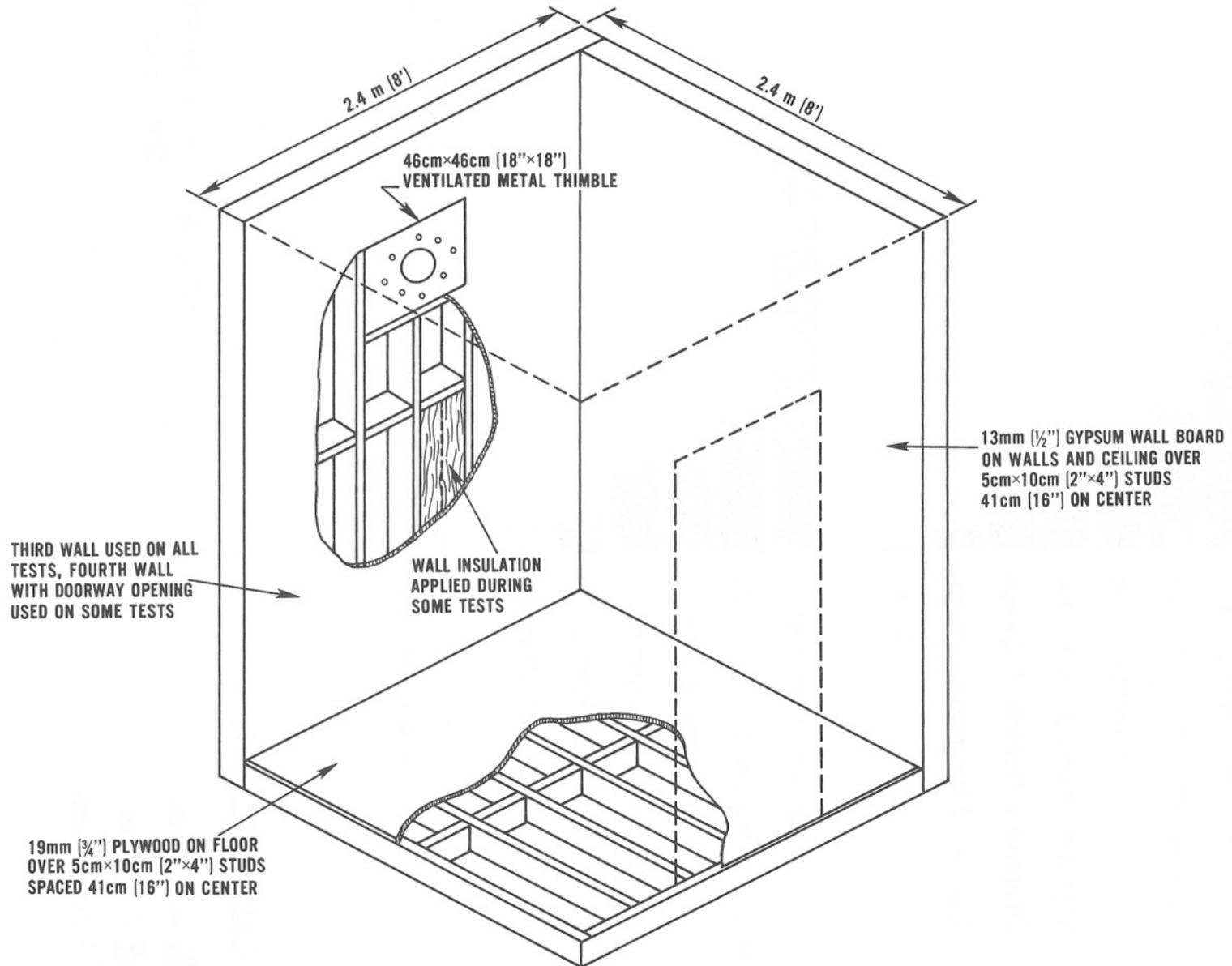
Figure 2. Construction of test enclosure used in room experiments.
