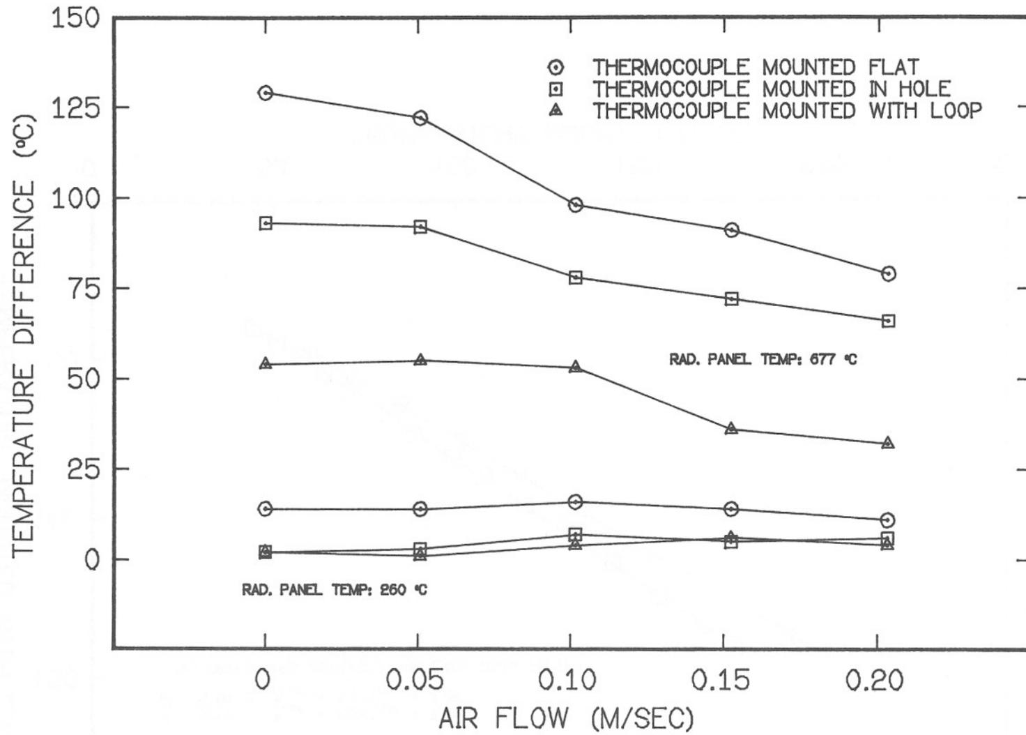
Figure 25. Surface/air temperature difference vs. airflow for different radiant panel temperatures.
