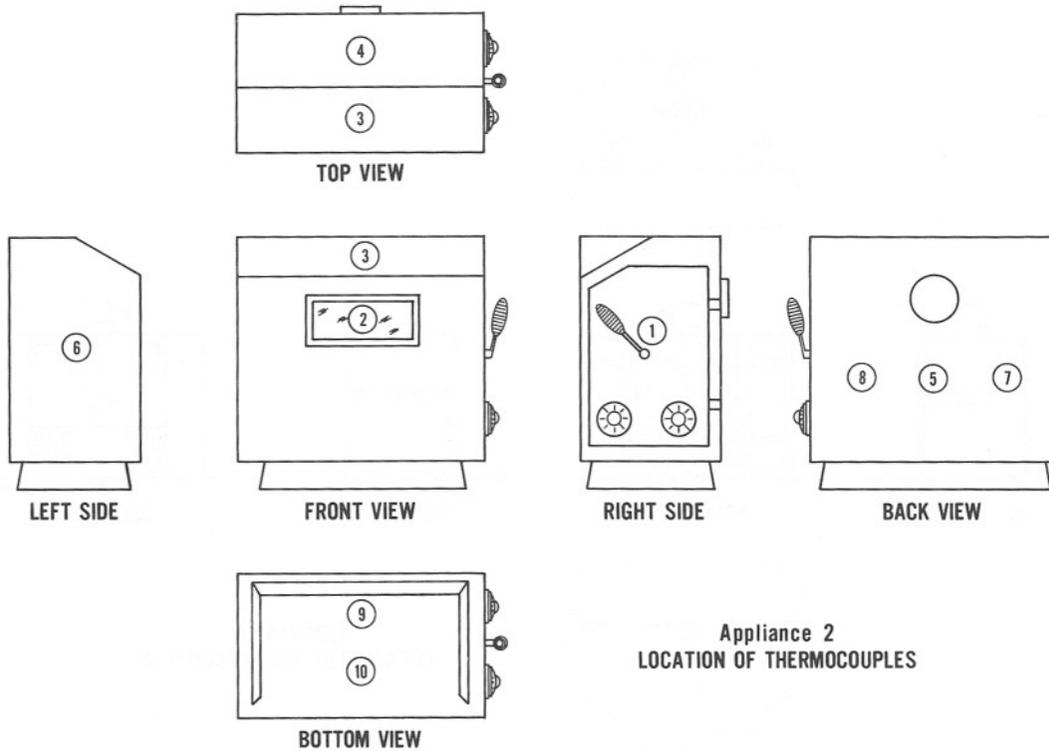
Figure 3. Instrumentation locations for appliance measurements in room experiments.
