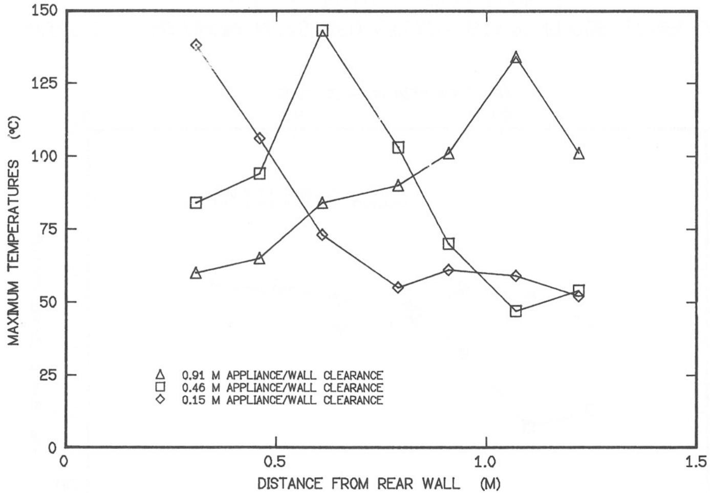
FIGURE 18: MAXIMUM MEASURED STEADY STATE FLOOR TEMPERATURES DURING TESTS OF APPLIANCE 4
