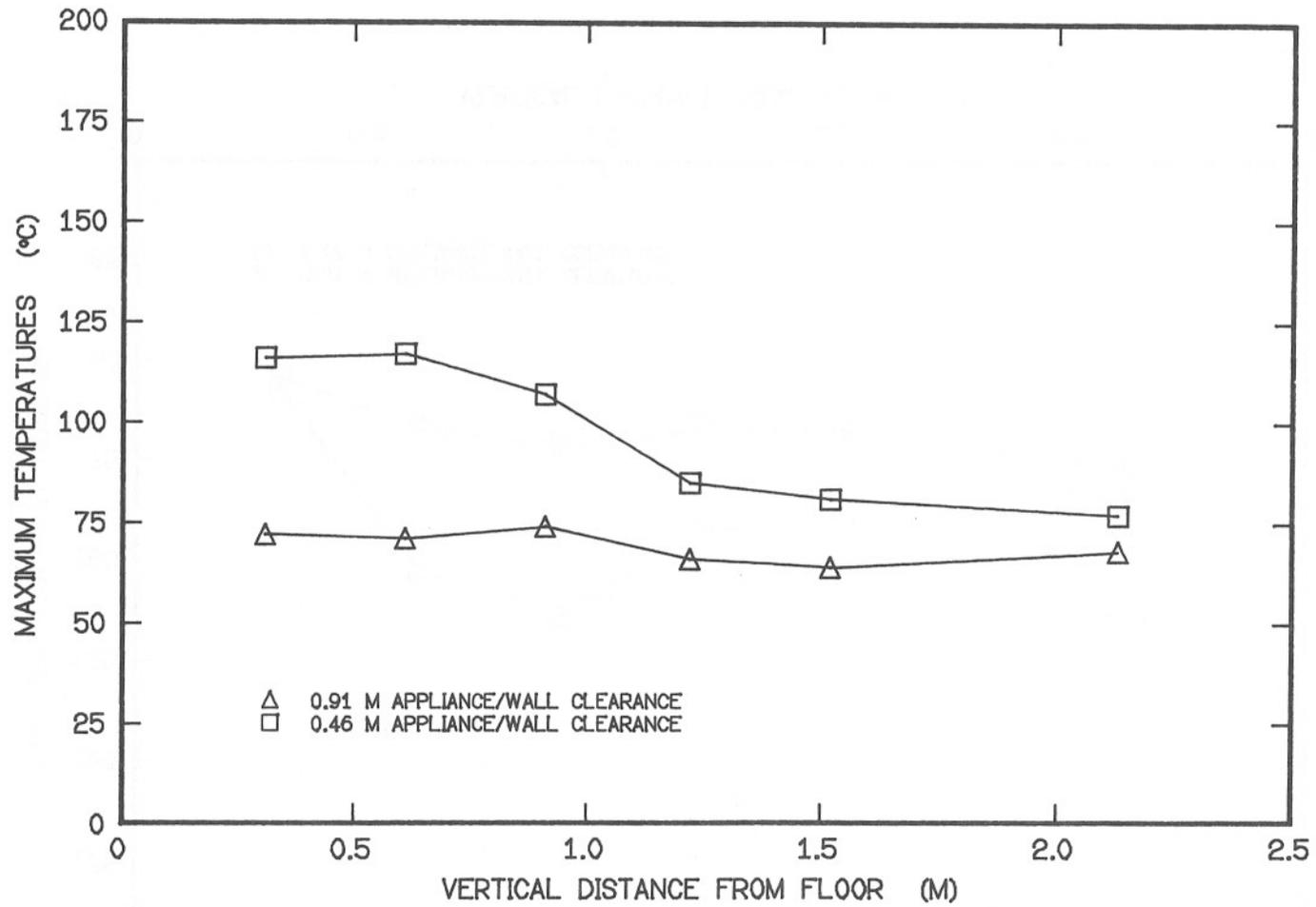
FIGURE 9: MAXIMUM MEASURED STEADY STATE WALL TEMPERATURES DURING TESTS OF APPLIANCE 2
