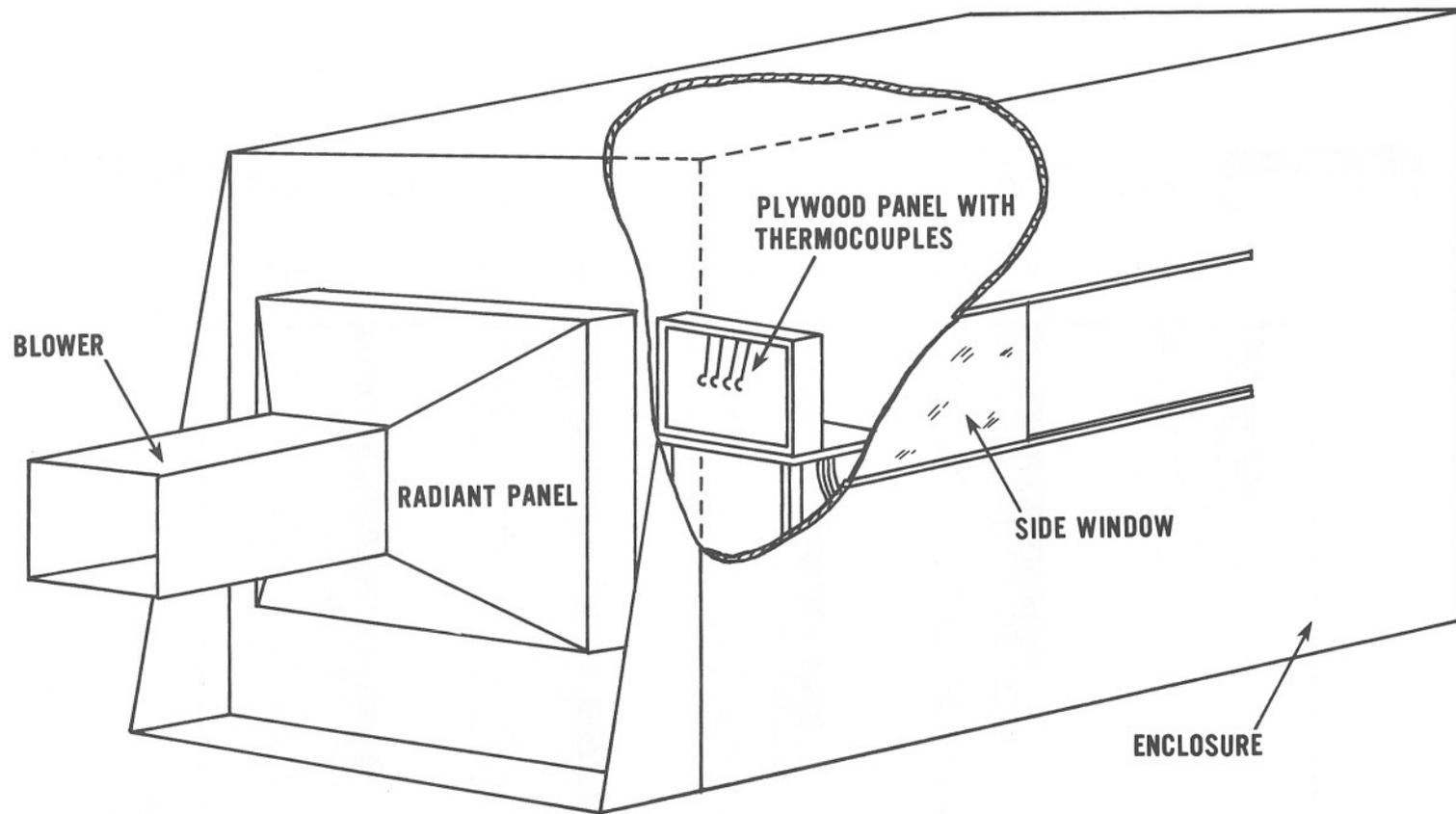
Figure 24. Test apparatus to evaluate thermocouple mounting techniques.
