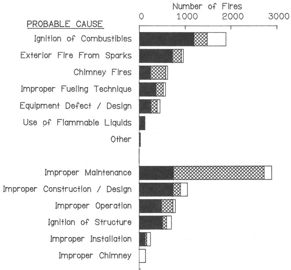
Figure 1: Breakdown of fire incidents by probable cause and equipment type as recorded in NFIRS fire incident data
