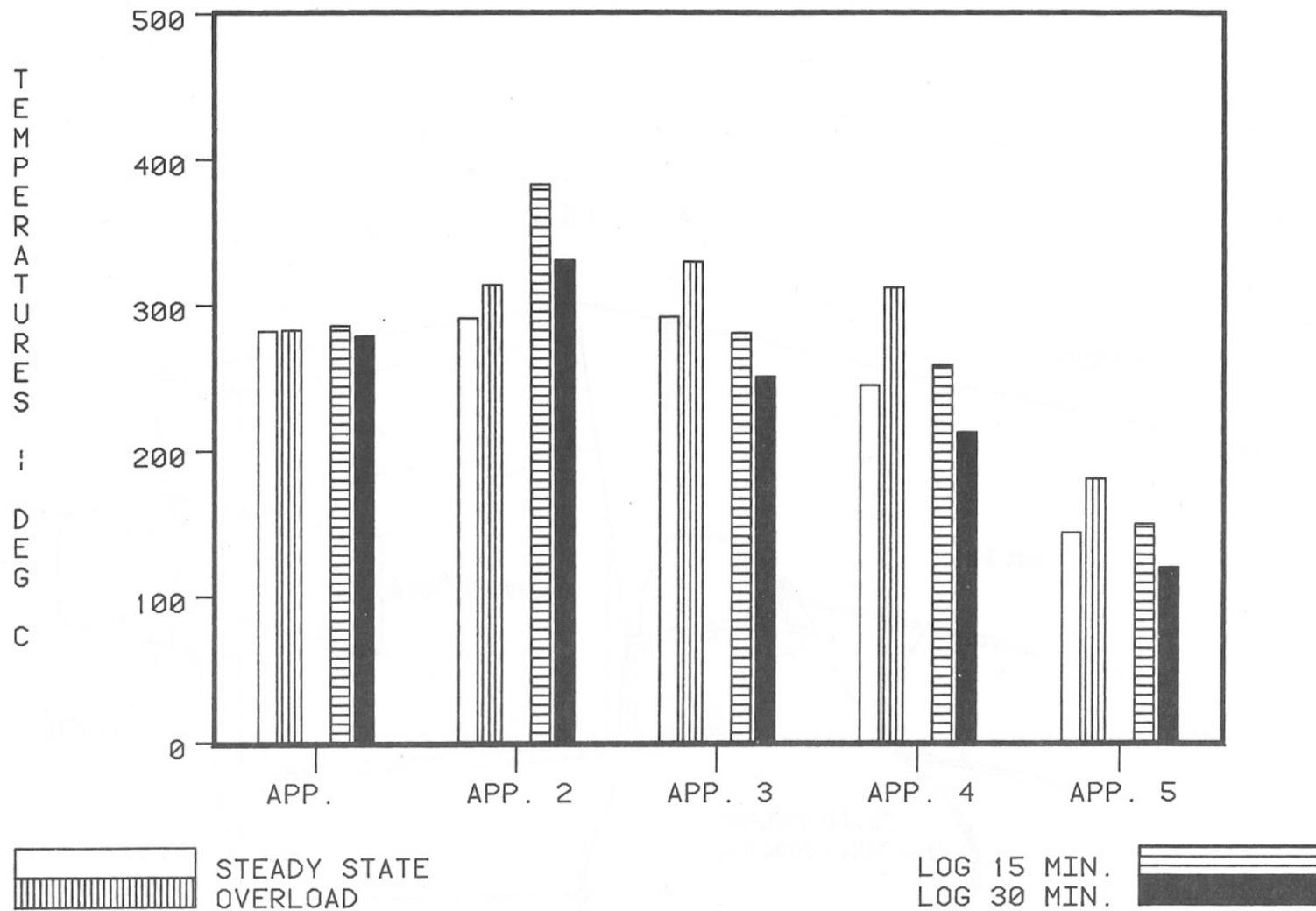
Figure 23. A comparison of maximum appliance temperatures for tests using logs as a fuel source with tests using douglas fir brands as a fuel source.
