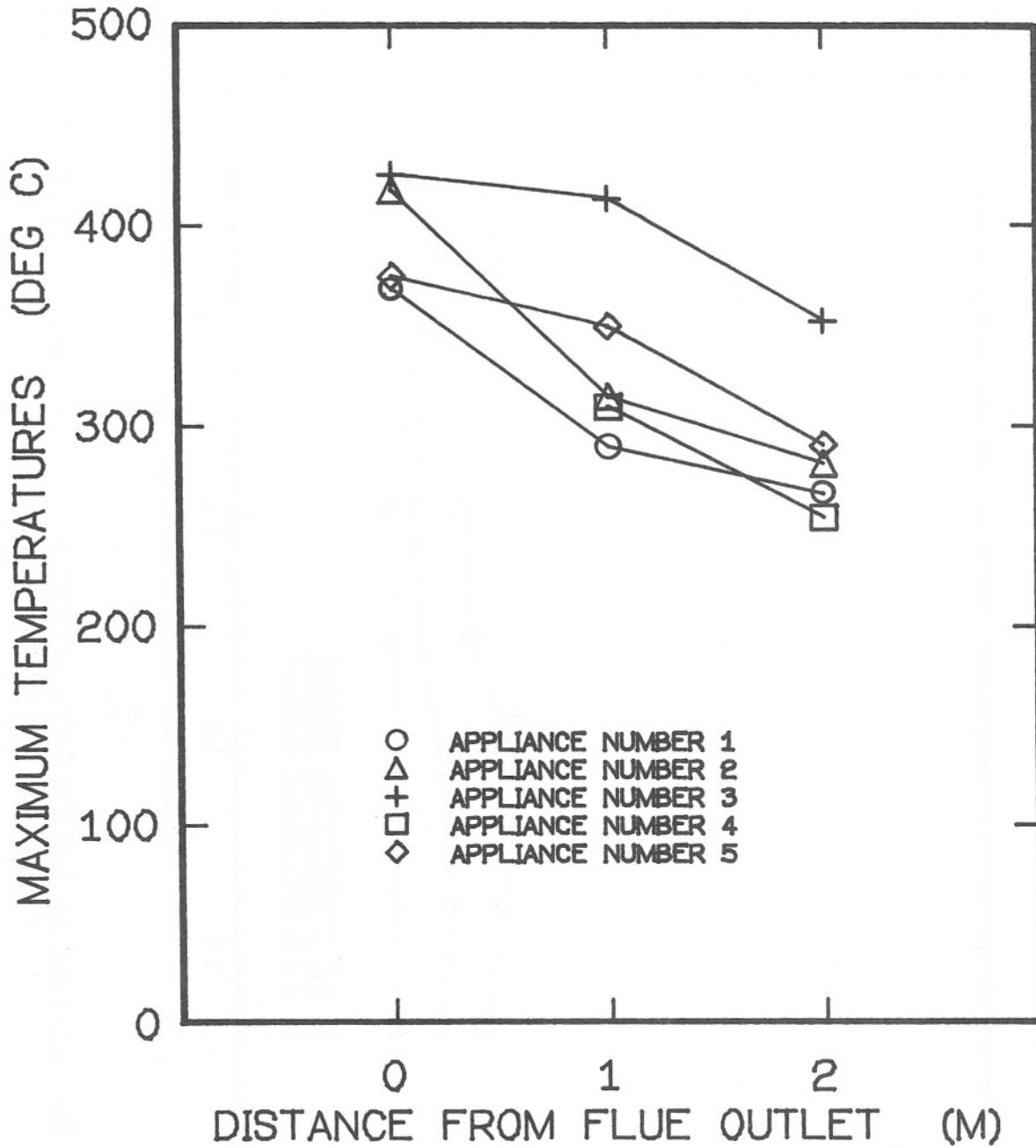
Figure 7. Flue pipe surface temperatures measured during tests of several wood-burning appliances.
