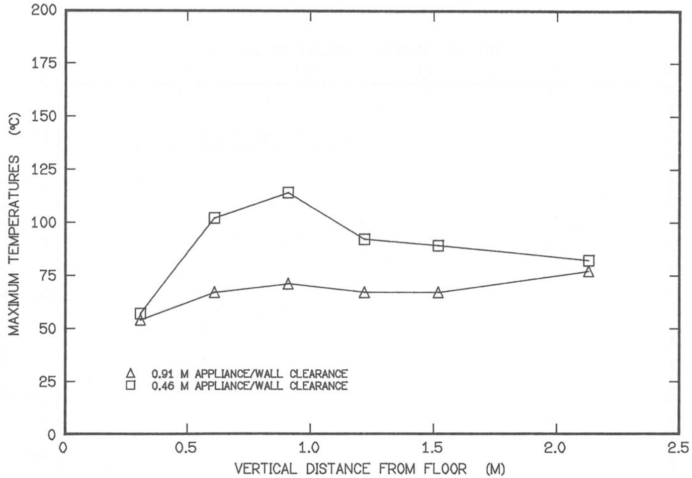
FIGURE 10: MAXIMUM MEASURED STEADY STATE WALL TEMPERATURES DURING TESTS OF APPLIANCE 3
