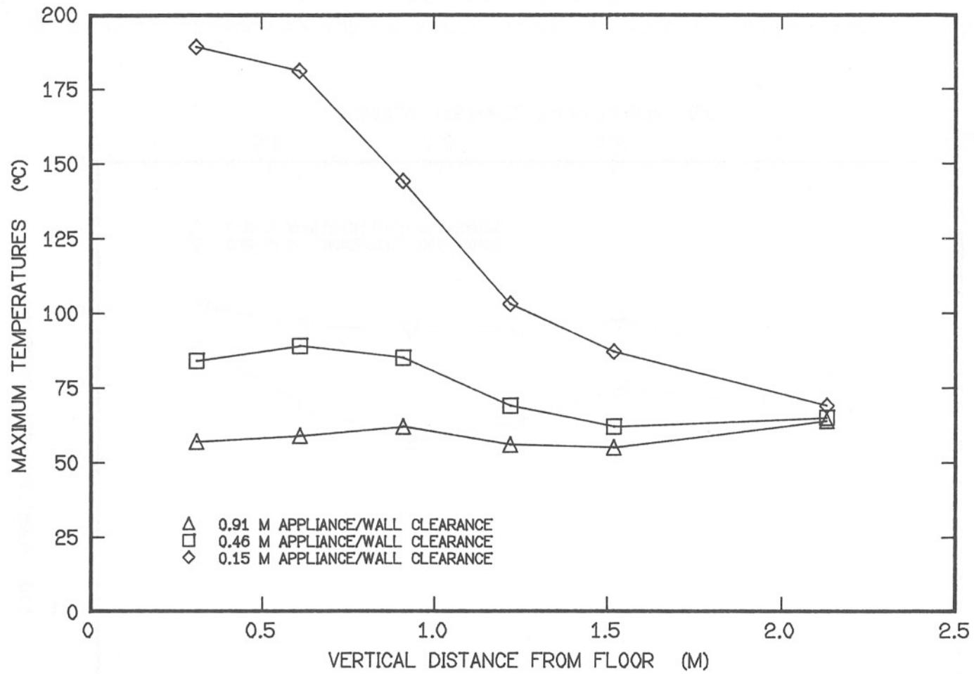
FIGURE 11: MAXIMUM MEASURED STEADY STATE WALL TEMPERATURES DURING TESTS OF APPLIANCE 4
