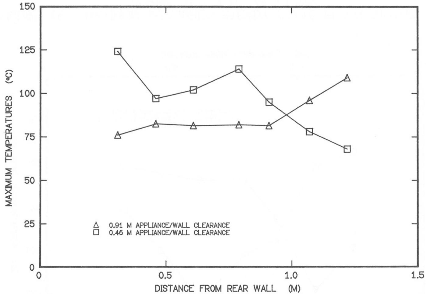
FIGURE 20: MAXIMUM MEASURED STEADY STATE FLOOR TEMPERATURES DURING TESTS WITH WALL INSULATION
