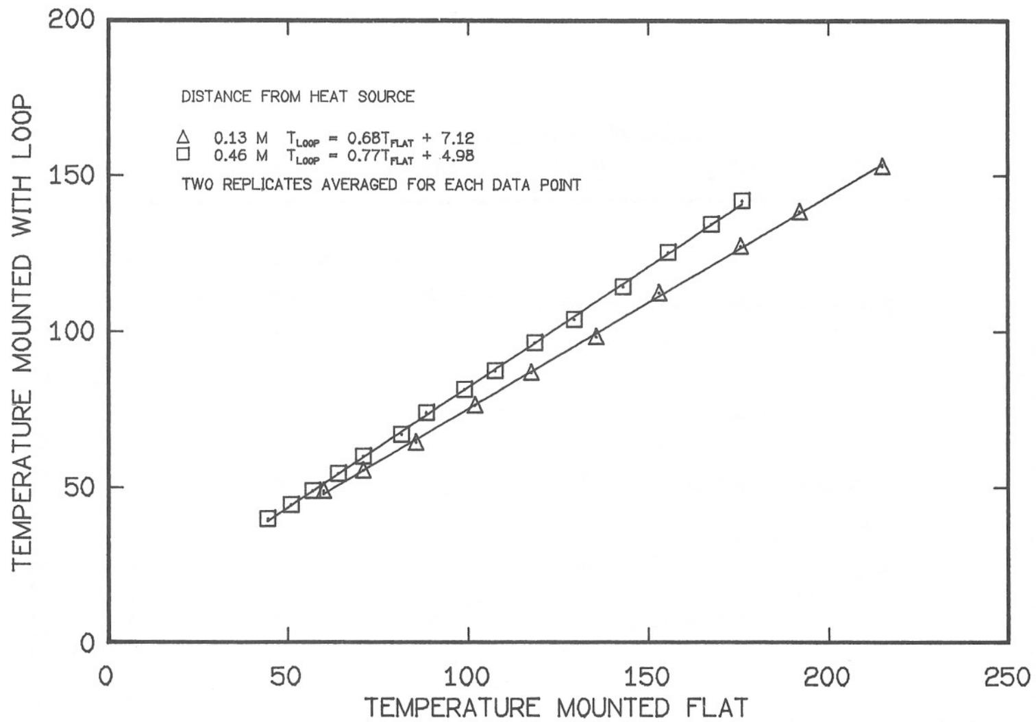
Figure 26. Surface temperatures as measured using different thermocouple mounting techniques.
