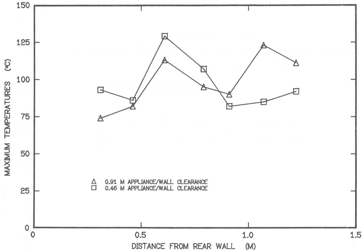
FIGURE 16: MAXIMUM MEASURED STEADY STATE FLOOR TEMPERATURES DURING TESTS OF APPLIANCE 2
