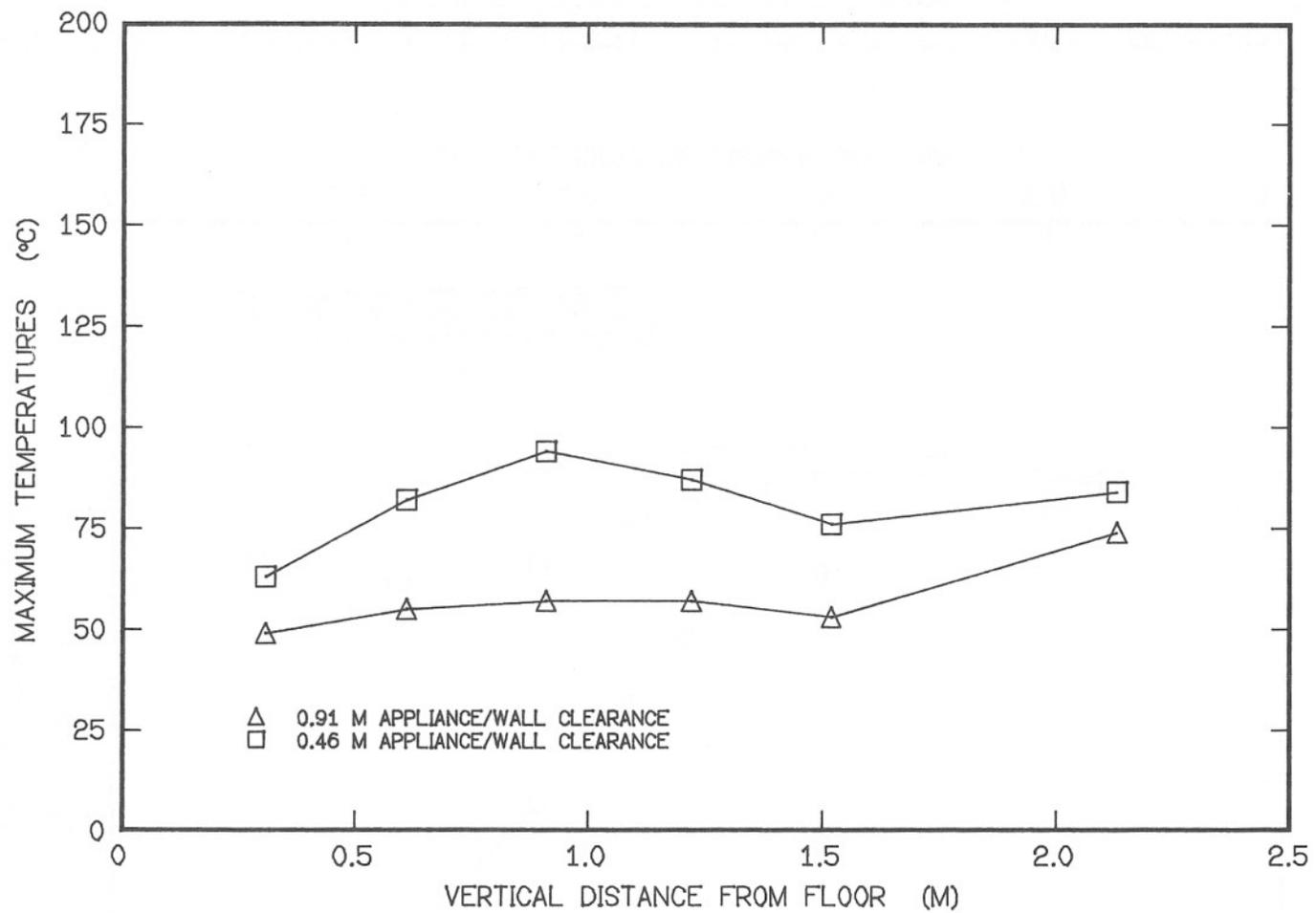
FIGURE 12: MAXIMUM MEASURED STEADY STATE WALL TEMPERATURES DURING TESTS OF APPLIANCE 5
