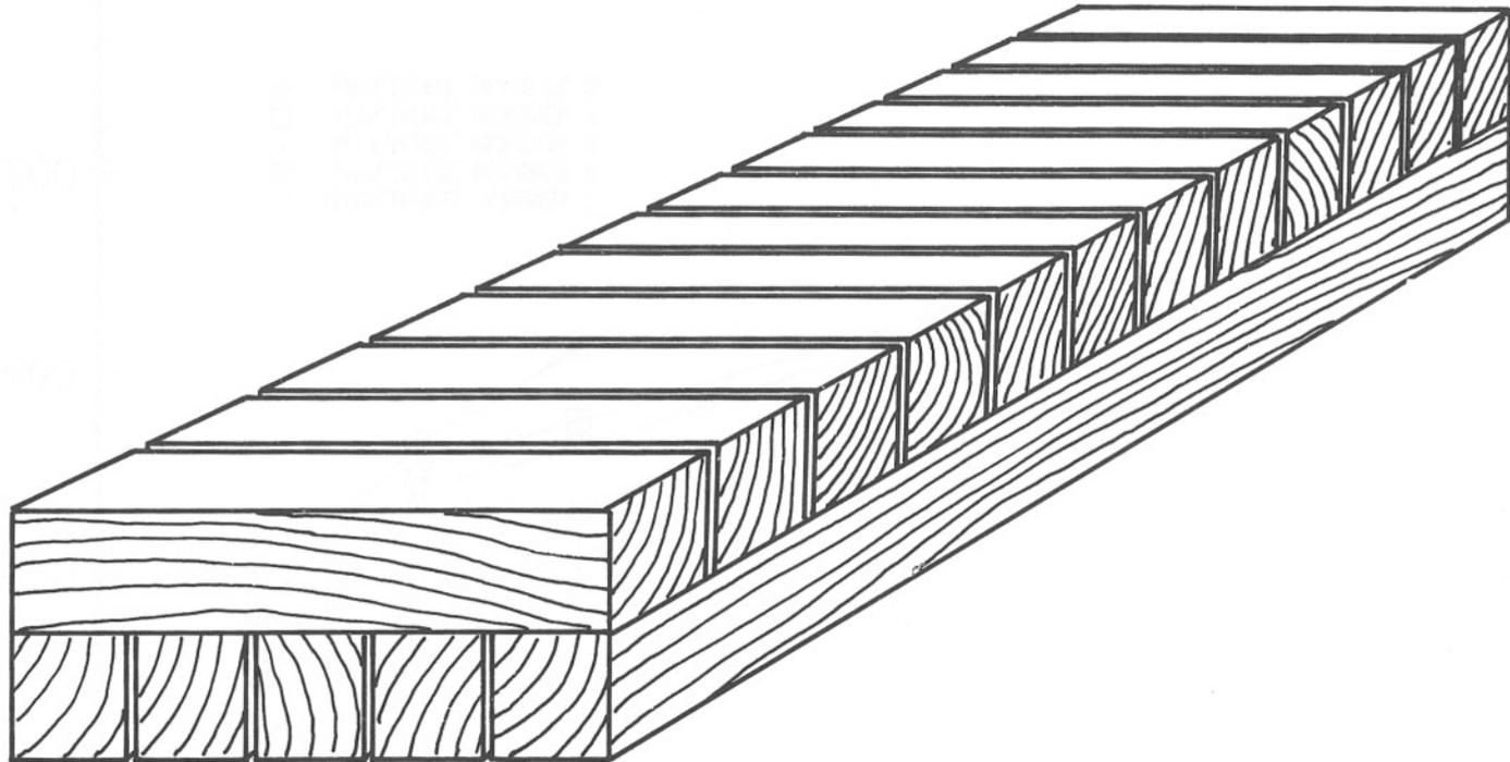
Figure 5. Construction of "brands" used in room experiments.
