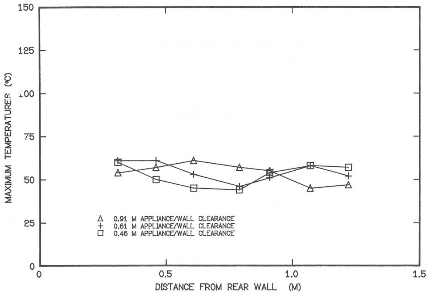
FIGURE 15: MAXIMUM MEASURED STEADY STATE FLOOR TEMPERATURES DURING TESTS OF APPLIANCE 1
