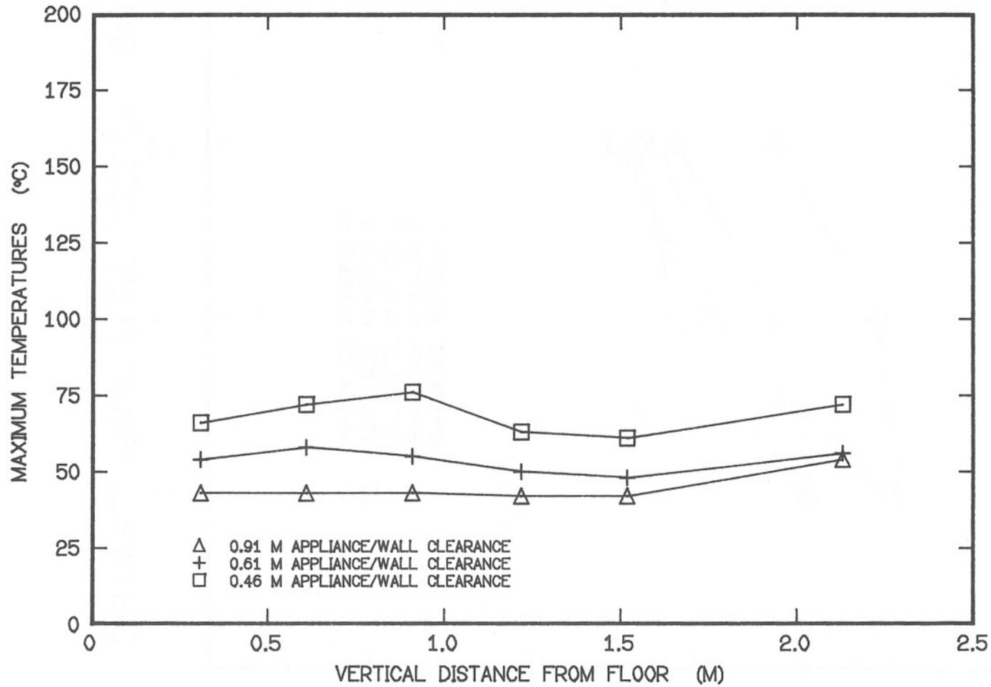
FIGURE 8: MAXIMUM MEASURED STEADY STATE WALL TEMPERATURES DURING TESTS OF APPLIANCE 1
