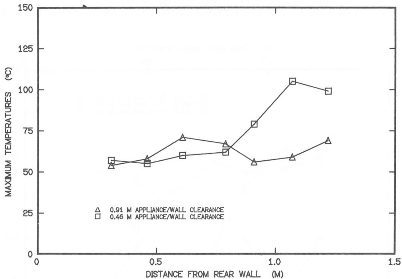
FIGURE 17: MAXIMUM MEASURED STEADY STATE FLOOR TEMPERATURES DURING TESTS OF APPLIANCE 3
