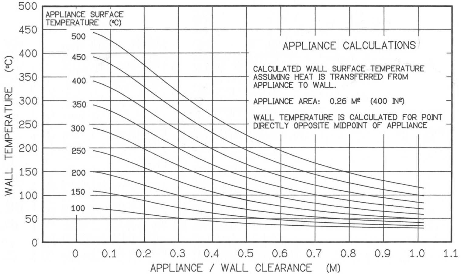
FIGURE 29: PREDICTED WALL SURFACE TEMPERATURE FOR HEAT TRANSFER FROM APPLIANCE ONLY
