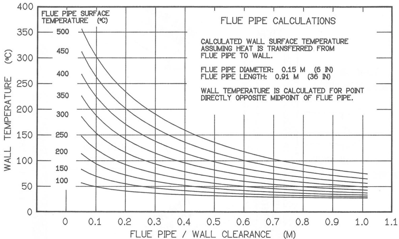
FIGURE 28: PREDICTED WALL SURFACE TEMPERATURE FOR
