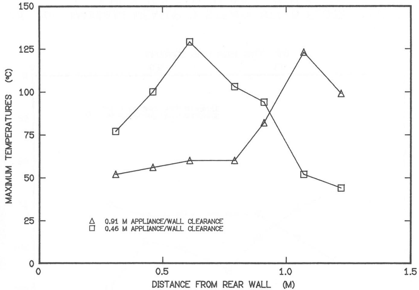
FIGURE 19: MAXIMUM MEASURED STEADY STATE FLOOR TEMPERATURES DURING TESTS OF APPLIANCE 5
