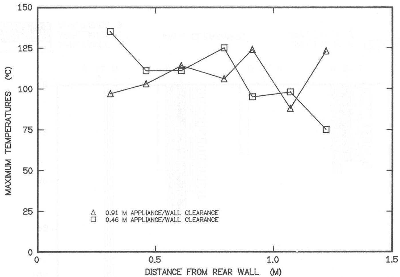
FIGURE 21: MAXIMUM MEASURED STEADY STATE FLOOR TEMPERATURES DURING TESTS WITH FRONT WALL
