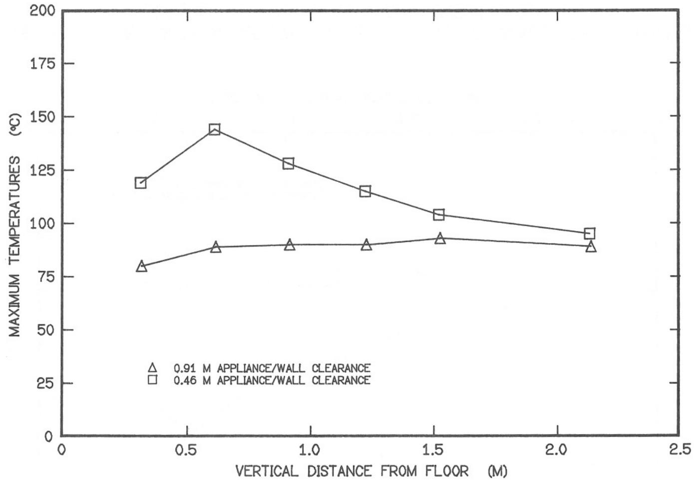
FIGURE 14: MAXIMUM MEASURED STEADY STATE WALL TEMPERATURES DURING TESTS WITH FRONT WALL
