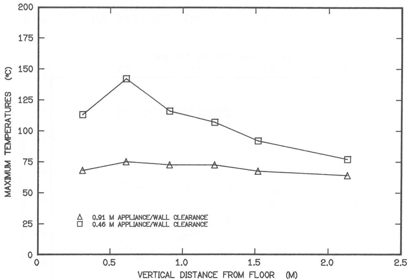
FIGURE 13: MAXIMUM MEASURED STEADY STATE WALL TEMPERATURES DURING TESTS WITH WALL INSULATION
