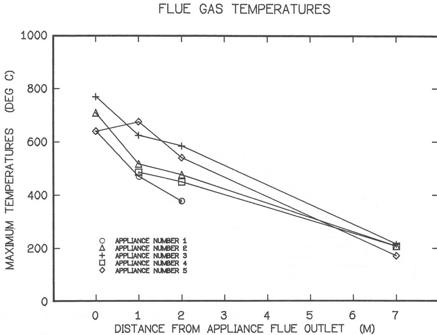
Figure 6. Flue gas temperatures measured during tests of several wood-burning appliances.
