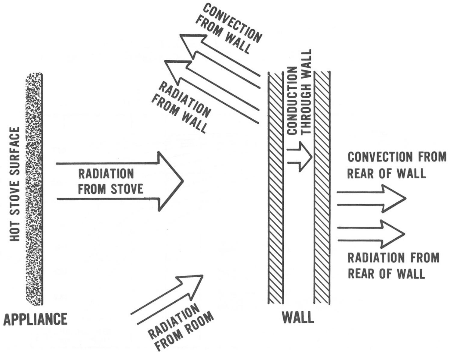
Figure 27. Heat transfer to wall surfaces.
