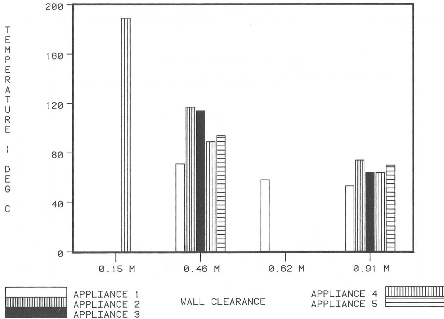
Figure 22. Effect of appliance/wall clearance on measured wall temperatures during tests of several wood-burning appliances.
