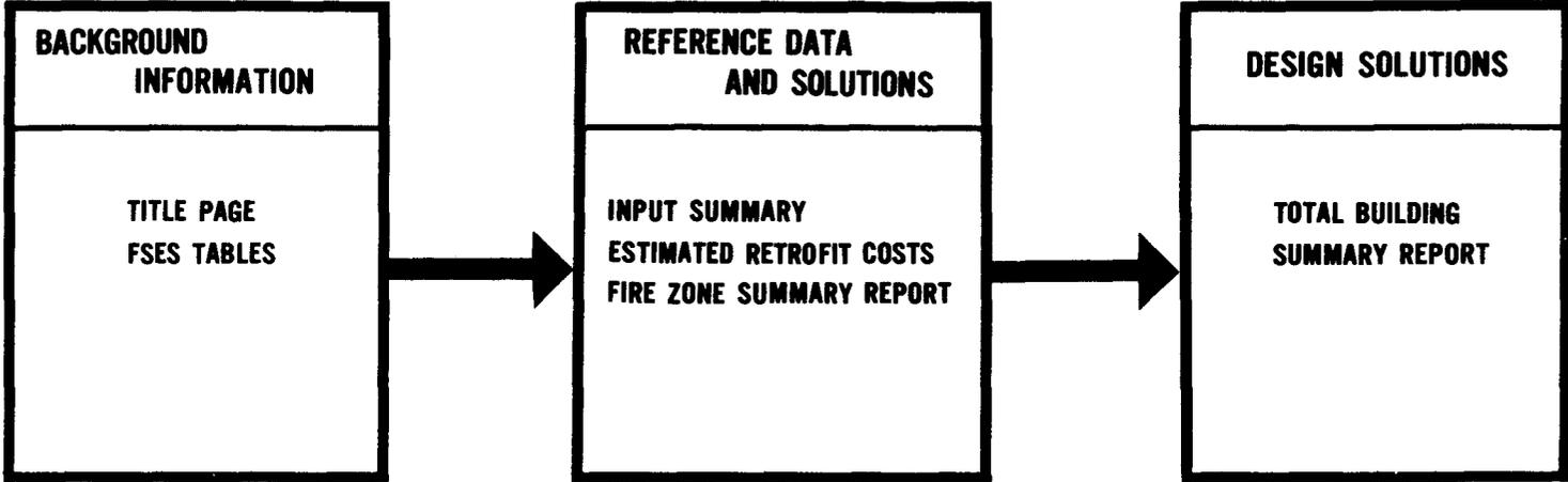
Figure 3.2 Outputs of the FSESCM Computer Program
