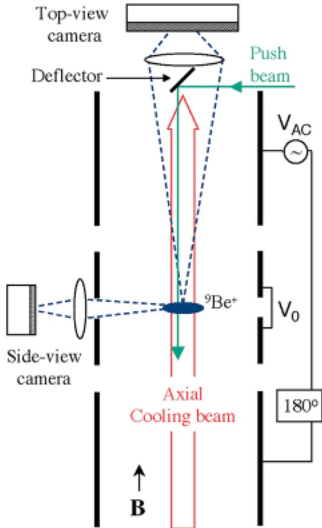
Fig. 1. The cylindrical experimental apparatus and its optical diagnostics. In this work  $B = 4.46$  T and  $V_0$  ranged from  $-1$  kV to  $-2$  kV.
