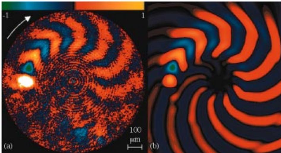
Fig. 2. Top-view images of the differential intensities, proportional to the ion velocities, induced by a laser push beam (white spot) incident on a disk-shaped ion plasma rotating clockwise. (a) shows experimental results while (b) shows the prediction from theory.
