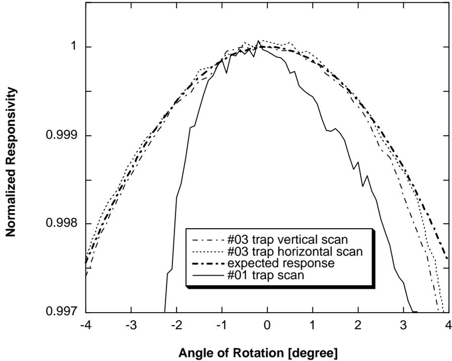
Fig. 7. Irradiance mode angular responses of tunnel-trap radiometers using 3.5 mm diameter apertures. The experimental #01 trap was built with six equal size photodiodes. The beam was clipped on the sixth (last) photodiode. The horizontal and vertical angular response scans of the optimized tunnel-trap radiometer #03 are very close to the expected cosine response within an angular range of 5°.
