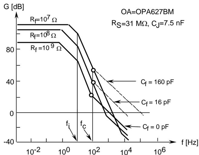
Fig. 8. Calculated loop gain characteristics of trap-radiometer #03 for the highest three signal-gains. The open-loop gain roll-off frequency of the operational amplifier is  $f_i$ . The dashed
