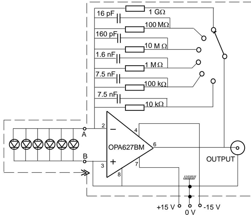
Fig. 9. Circuit diagram of the tunnel-trap radiometer.
