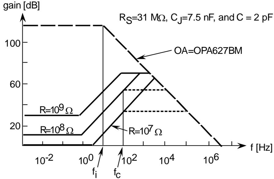
Fig. 11. Calculated voltage gain characteristics of the trap-radiometer. The open-loop gain roll-off frequency of the operational amplifier is  $f_i$ . The short dashed lines show the effect of the partial frequency compensations at frequency  $f_c$ .
