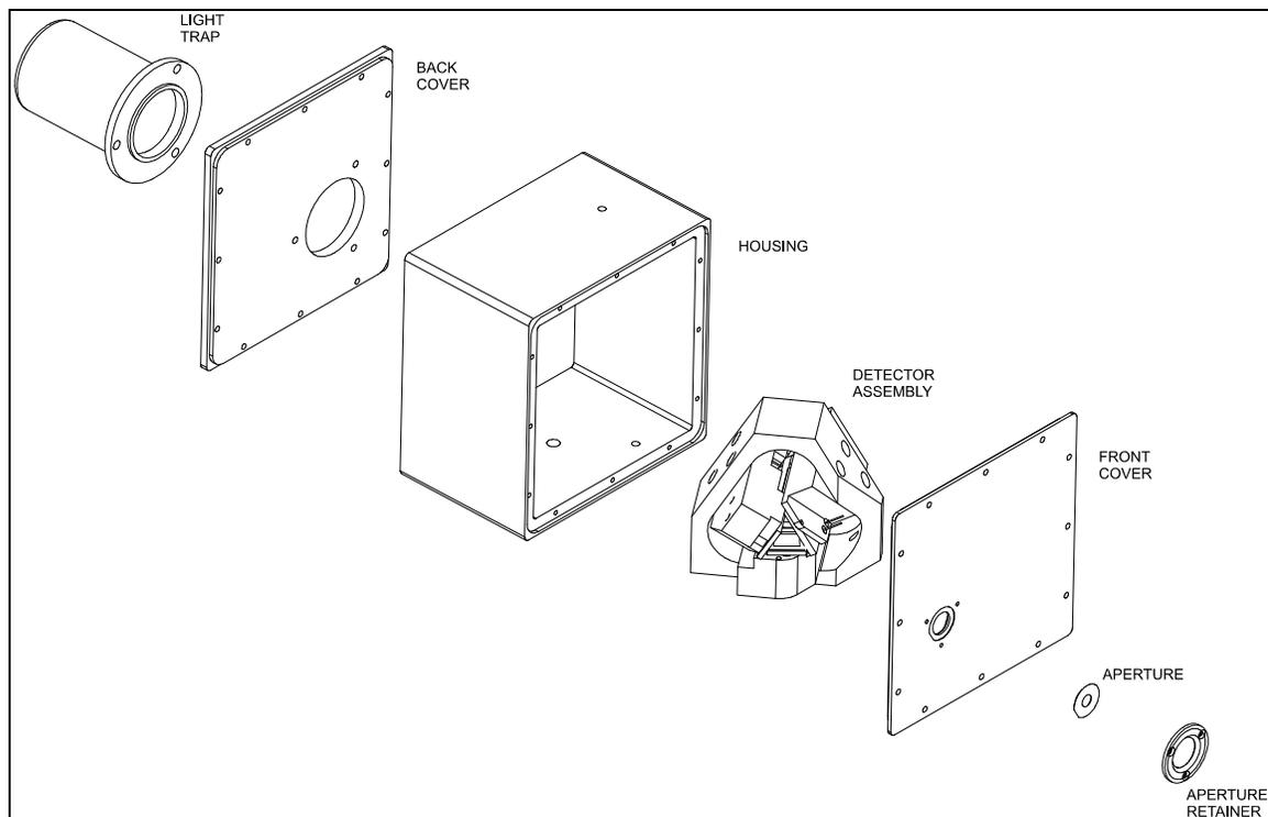
Fig. 6. Exploded view of the triangular tunnel-trap radiometer.
