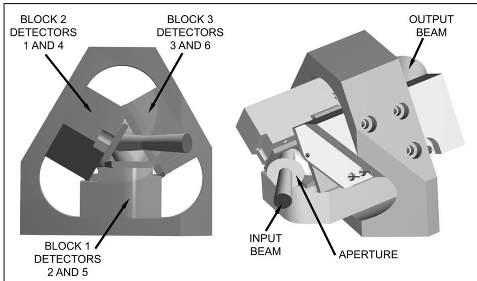
Fig. 5. Construction of the triangular tunnel-trap detector holder
