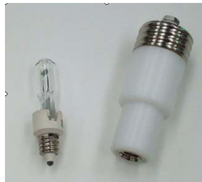
Figure 2. Photograph of a 75 W miniature QTH transfer standard lamp and an E26 screw base adapter.
