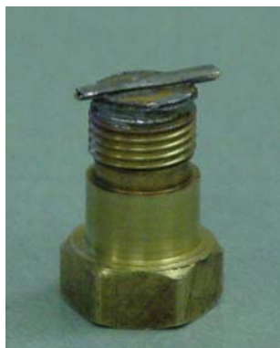
Figure 6.19 Oil Capsule Top Connected to Flow Restrictor
