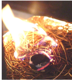
Fig. 4 Single flaming ember which produced flaming ignition in a pine needle bed held at 11% moisture, d_0 = 25 mm.
