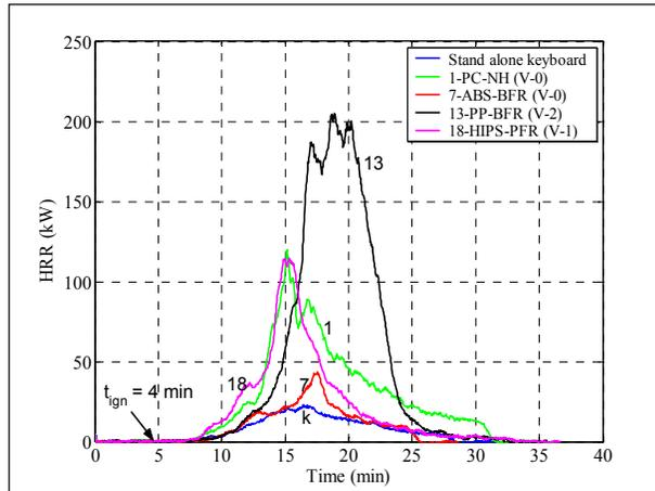
Figure 5. HRR curves for keyboard ignition of 19" computer monitors.
