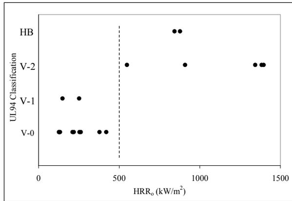
Figure 2. Comparison of UL94 ranking and intrinsic HRR for 3.2 mm specimens.
