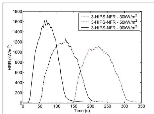
Figure 1. HRR curves for 3-HIP-NFR (UL94 HB) 3.2 mm sample thickness.
