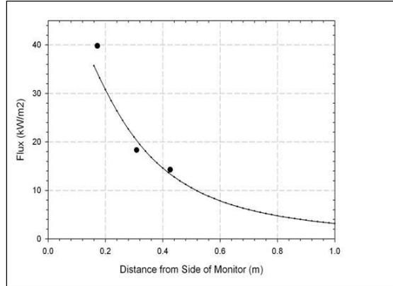
Figure 8. View-factor based extrapolation curve and flux measurements from keyboard ignition of 1-PC-NH monitor.
