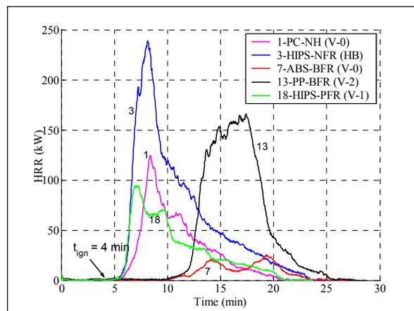
Figure 6. HRR curves for radiant heat panel “forced ignition” of 19” monitors.
