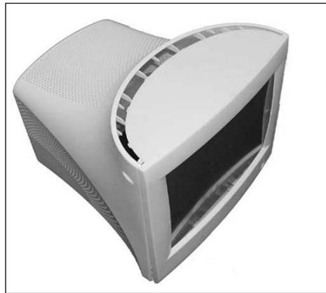
Figure 3. 19" Computer monitor specimen used in full-scale testing.
