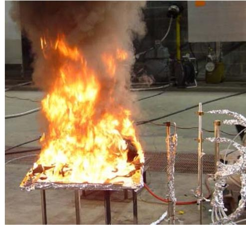
Figure 4. Heat release rate curves for needle flame ignition of 19" monitors. Ignition flame applied to specimen at  $t = 4$  min. Image of monitor test, 3-HIPS-NFR, near peak heat release rate (right). Array of heat flux gauges is shown on right side of image
