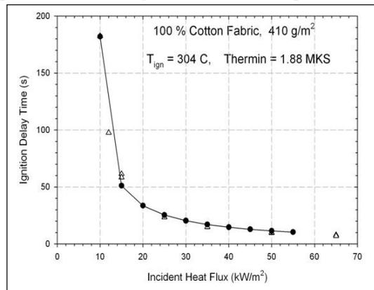
Figure 7. Radiative ignition of cotton fabric in the Cone Calorimeter.
