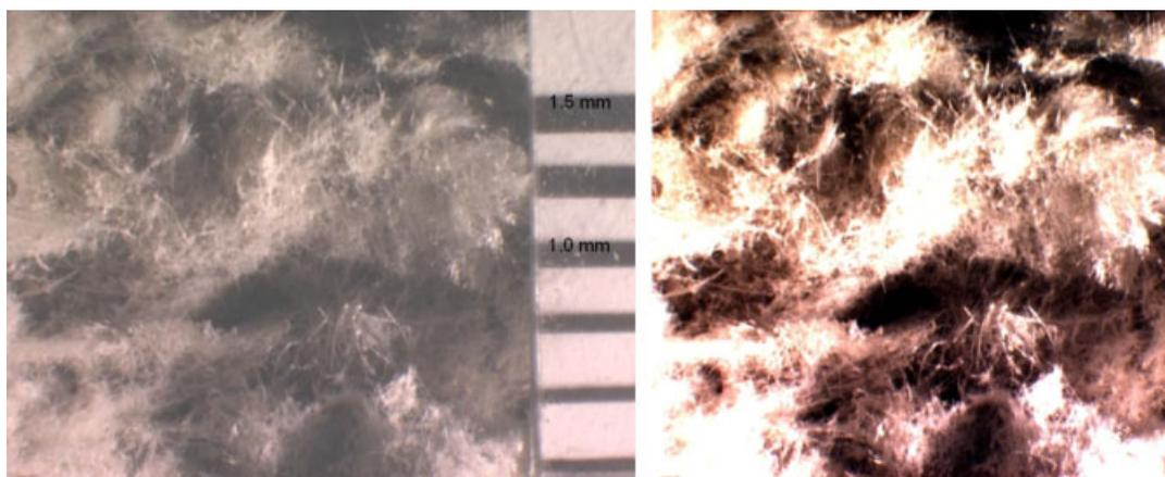
Figure 7. Optical micrograph for portland-cement-based spray-applied FRM-B. Typical pore *diameter* as indicated by the labelled scale bars in the middle of the two images is on the order of 1.5 mm corresponding to a pore radius of 0.75 mm. The original image is on the left and a contrast-enhanced version that better highlights the porosity is shown on the right.
