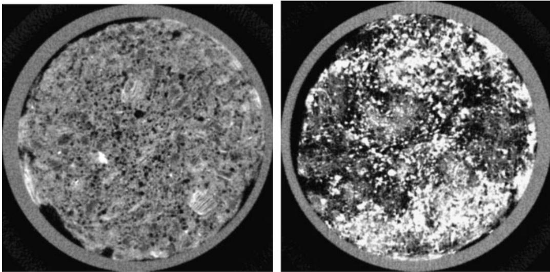
Figure 9. Examples of two-dimensional images from three-dimensional microtomography data sets for gypsum-based (left) and mineral fibre/portland-cement-based (right) FRMs. Materials were imaged in a polypropylene tube with a nominal inner diameter (ID) of 27 mm.
