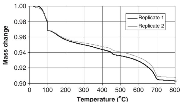
Figure 2. Example thermogravimetric results for a portland-cement-based spray-applied FRM with a heating rate of 5°C/min. Results are given for two nominally identical  $\approx 50$  mg replicates. Maximum observed COV for mass loss between the two replicate samples is 0.4%.
