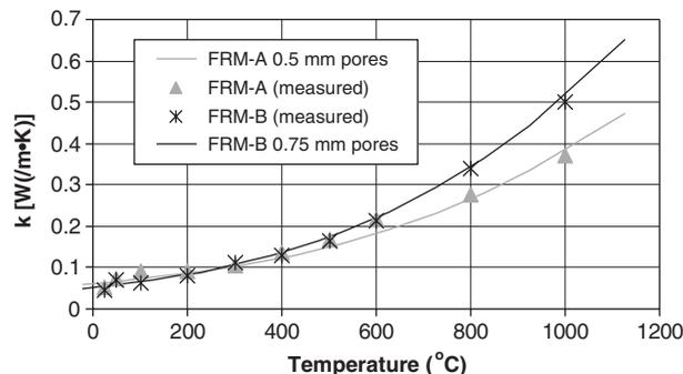
Figure 4. Measured thermal conductivities [1] and predictions based on theory of Russell/Loeb [11, 14] for two similar portland-cement based spray-applied FRMs.
