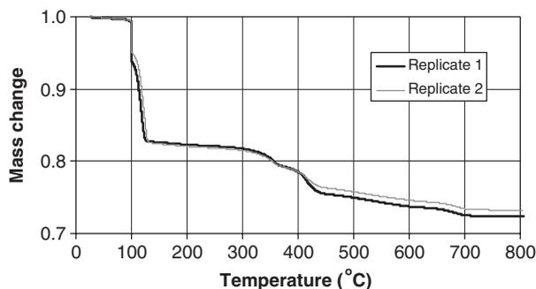
Figure 1. Example thermogravimetric results for a gypsum-based spray-applied FRM with a nominal heating rate of  $5^{\circ}\text{C}/\text{min}$ . Results are for two nominally identical  $\approx 50$  mg replicates. Maximum observed coefficient of variation (COV) for mass loss between the two replicate samples is 0.9%.
