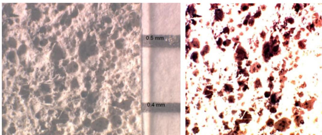
Figure 8. Optical micrograph for gypsum-based spray-applied FRM-C. Typical pore *diameter* as indicated by the labelled scale bars in the middle of the images is on the order of 0.4 mm corresponding to a pore radius of 0.2 mm. The original image is on the left and a contrast-enhanced version that better highlights the porosity is shown on the right.
