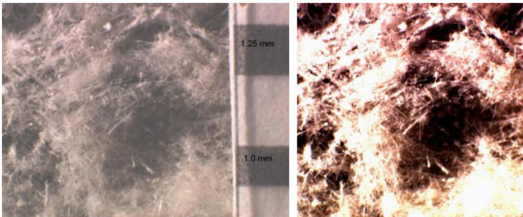
Figure 6. Optical micrograph for portland-cement-based spray-applied FRM-A. Typical pore diameter as indicated by the labelled scale bars in the middle of the two images is on the order of 1.0 mm corresponding to a pore radius of 0.5 mm. The original image is on the left and a contrast-enhanced version that better highlights the porosity is shown on the right.
