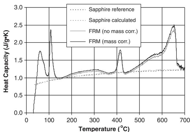
Figure 3. Example DSC results (original and mass corrected) for a portland-cement-based spray-applied FRM using gold pans and a sapphire reference.
