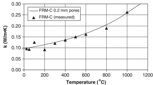
Figure 5. Measured thermal conductivities [1] and predictions based on theory of Russell/Loeb [11, 14] for a gypsum-based spray-applied FRM.
