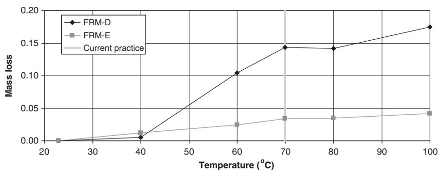
Figure 10. Mass loss (fraction) upon long term (two to three months) oven exposure to different temperatures for gypsum-based (FRM-D) and portland-cement-based (FRM-E) FRMs (sample size of  $\approx 3$  g).
